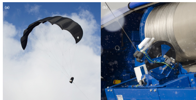
Figure 1. AWE system with (a) the 25 m 2 V3.25B kite and (b) the 100 kW ground station in operation in 2018 (photos courtesy of Kitepower B.V.).
