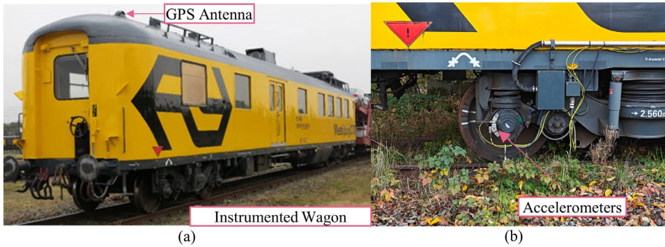
Figure 4.3: The ABA measurement system instrumented on the dedicated wagon: (a) a GPS antenna (source of photo: TU Delft OpenCourseWare), (b) accelerometers attached to an axle box.
