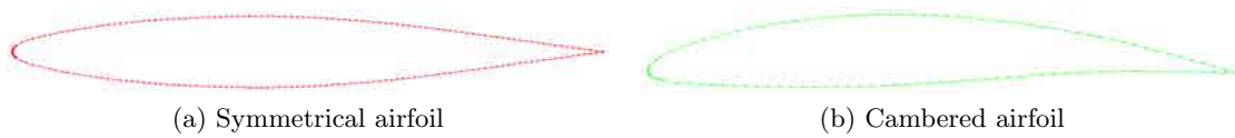
Figure 5.2: A symmetrical NACA - 65 1 (A)012 and highly cambered NACA - 64 1 (A)612 airfoil section used for the swept wing configurations.
