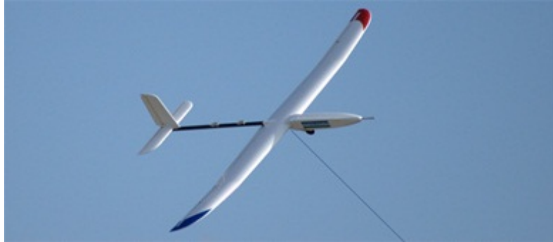
Figure 2.9: Prototype of the 10 kW PowerPlane design (from LabS55, 2011).
