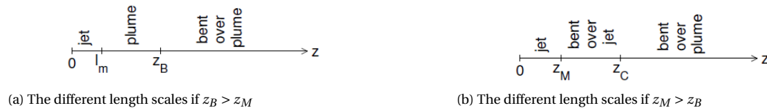
Figure C.1: The different length scales and flow regimes defining the sediment plume behaviour of a JICF [de Wit, 2015].
