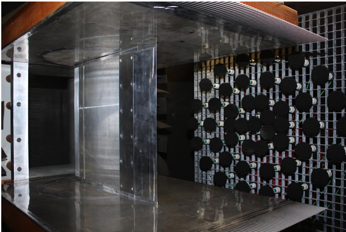
Figure 2. KAT set-up with microphone array and flat plate vertically mounted between the lined endplates.
