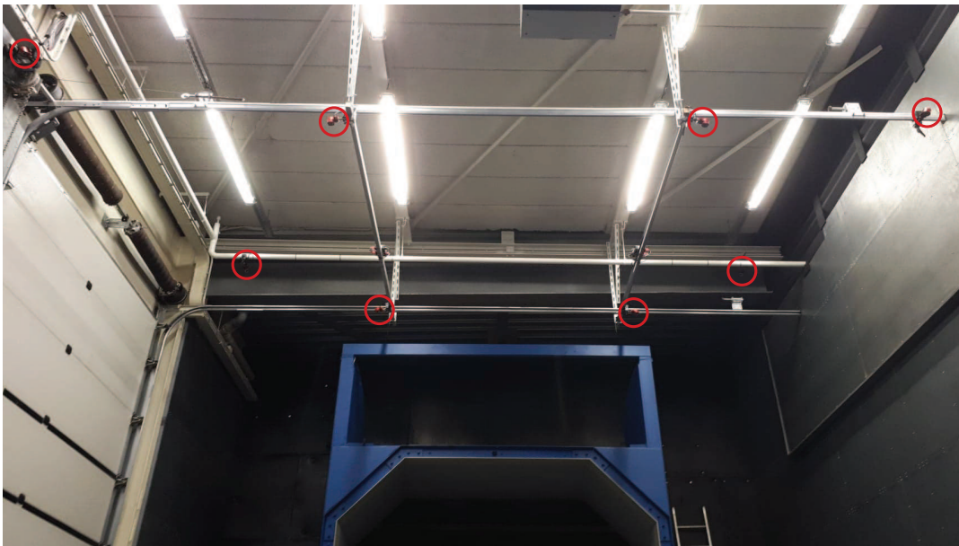
Figure A.1: Subset of the Flex 13 cameras installed on the ceiling of the OJF.
