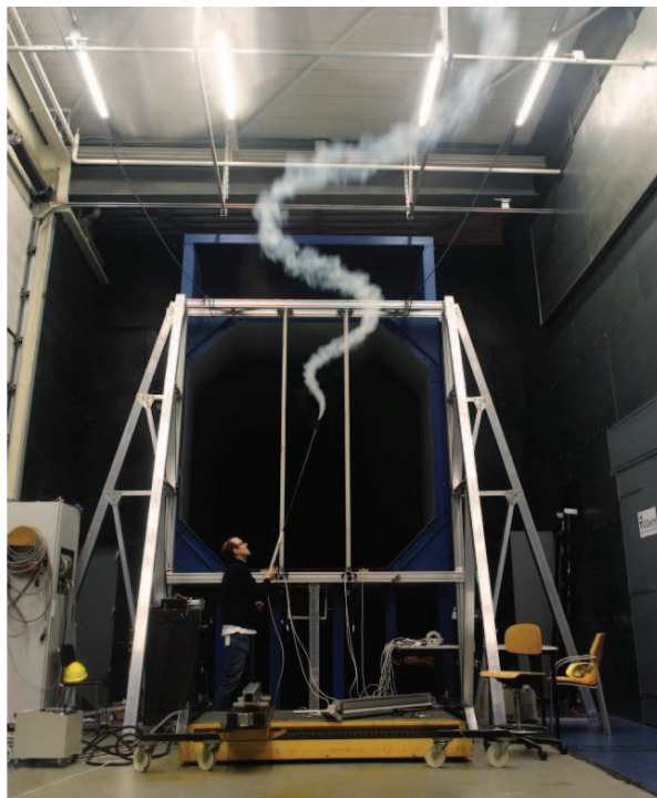
Figure 4.2: Gust generator inside the OJF producing a sinusoidal gust field in the flow (visualization by means of smoke). Reproduced from Lancelot et al. [2017b] .
