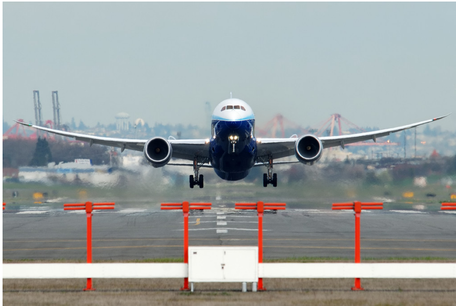
Figure 1.1: Boeing 787 at take-off showing the large flexibility of its wing. Reproduced from https://aviation.stackexchange.com/questions/14719/is-wing-flex-good (accessed: 13-11-2019).
