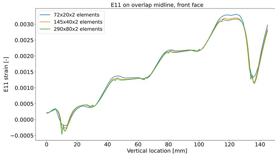
Figure D.3: Influence of increasing the number of finite elements, along the length and width of the plates, on the simulated surface strain distribution at the mid-line of the joint overlap. The legend specifies the number of elements used to represent the plates over the 40x40mm overlap area
