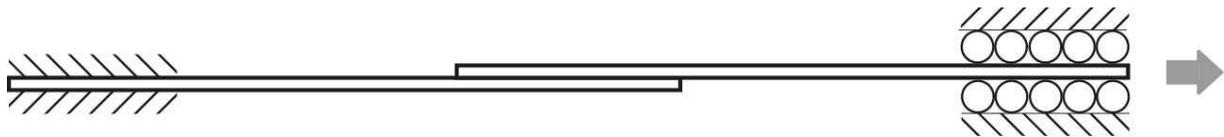
Figure 4.4: Sketch of real boundary conditions used for single weld spot testing in [15]. Picture courtesy of [15].
