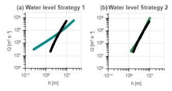
**Figure 11.** Discharge–water-level graphs for the recorded (black) and modelled discharge and stream levels with the optimal model performance ( $E_{\rm NS}$ ) using the Strickler–Manning equation for the discharge–stream-level conversion with cross-section information (**a**) extracted from Google Earth (Water level Strategy 1) or (**b**) obtained from a detailed field survey with an ADCP (Water level Strategy 2).
