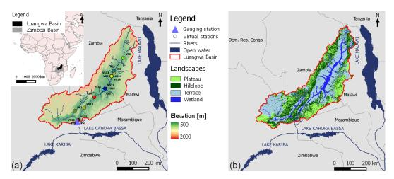
**Figure 1. (a)** Elevation map of the Luangwa River basin in Zambia including the Great East Road Bridges river gauging station and the locations of the 18 virtual stations (VS 1–VS 18; the red dot is VS 4) with altimetry data used in this study; their colours correspond to those in Fig. 4. **(b)** Map of the Luangwa River basin with the main landscape types (see Sect. 3.2).
