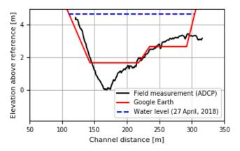
**Figure 5.** River cross section at Luangwa Bridge obtained from Google Earth and detailed field survey including the river water level on 2 June 2008. Field measurements were done with an Acoustic Doppler Current Profiler (ADCP) on 27 April 2018 at the coordinates 30°13′ E and 15°00′ S; the satellite image was taken on 2 June 2008. The reference level is equal to the lowest elevation level measured with the ADCP.
