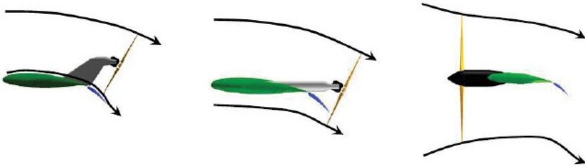
Figure 1.3: Three open rotor installation concepts on a wing. Arrows depict streamlines. Left: over-the-wing configuration. Center: Trailing-edge (or pusher) configuration. Right: Leading-edge (or tractor) configuration. [5]
