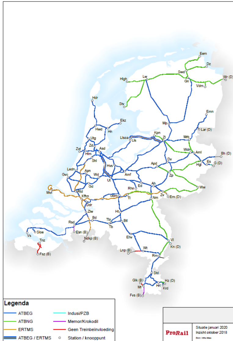
Figure 38 Automatic Train Protection systems in the Netherlands, green indicates ATBNG (ProRail, 2019a)
