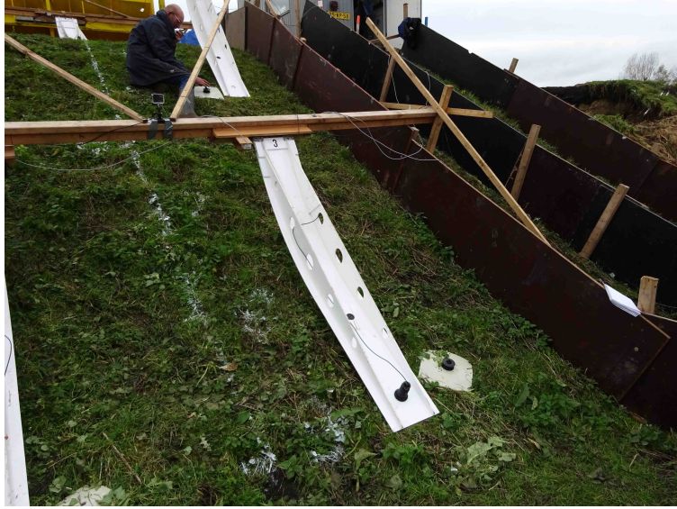
FIGURE 5.1: Both at the water surface and at the bottom the flow velocity was measured using a paddle wheel.
