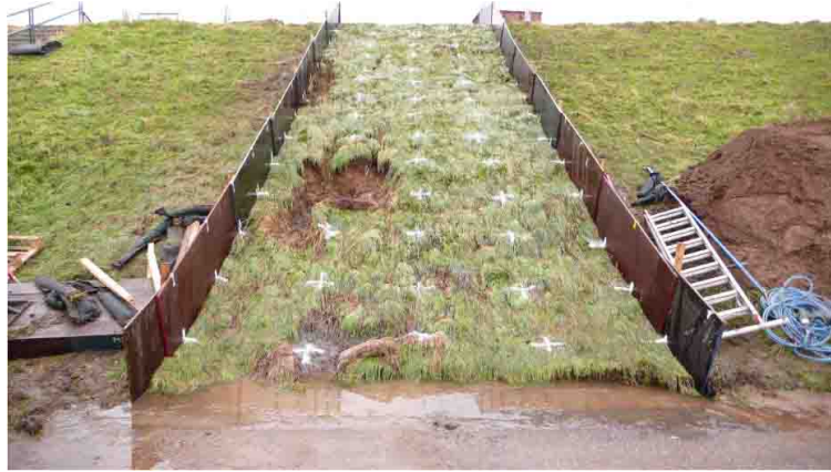
FIGURE 8.6: Tielrode overtopping experiment result test section 3, Picture from the factual report published by Flanders Hydraulics Research [22]
