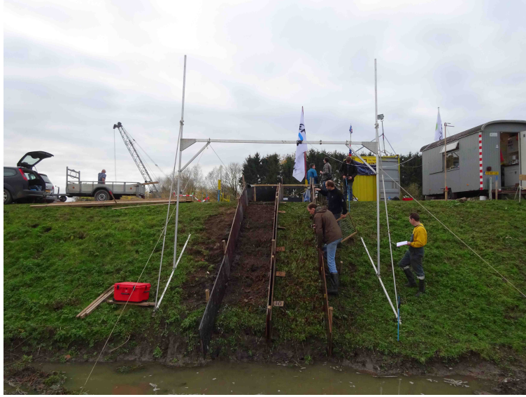
FIGURE 3.7: Second overflow test section. The section was split in half to create two parts: one to test on the grass layer and one to test directly on the clay layer.
