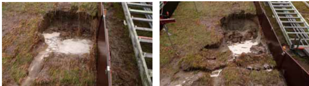
FIGURE F.6: Final result of the St Philipsland overtopping experiments. Photo taken by Infram B.V. [4]
