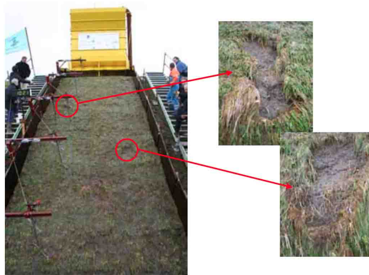
FIGURE F.5: Initial damage spots during the St Philipsland overtopping experiments. Photo taken by Infram B.V. [4]
