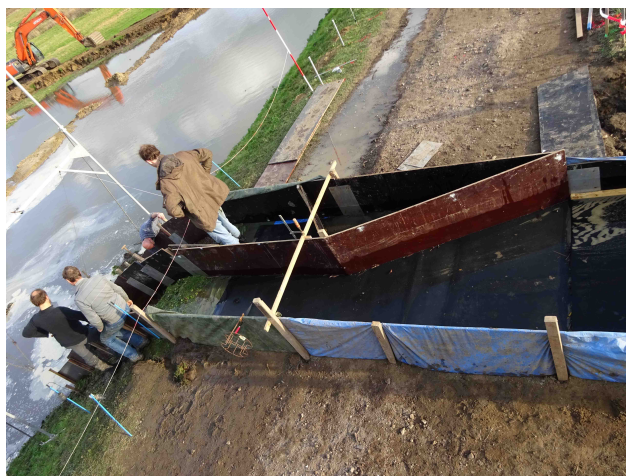
FIGURE 4.1: The first 3,5 m of the test section was covered with a plastic sheet to prevent erosion on the crest. Therefore the grass cover was exposed only just in front of the land side slope.
