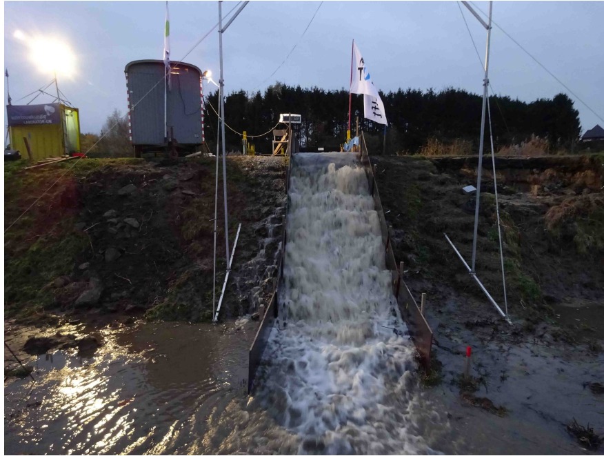
FIGURE 4.6: Overflow test at 85 \text{ lm}^{-1}\text{s}^{-1} . Although not clearly visible on the picture, the right part of the test section appeared to be more aerated than the left part.
