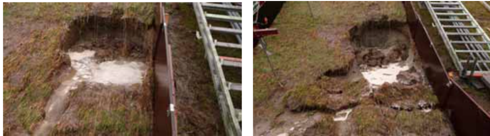
FIGURE 8.12: Final result of the St Philipsland overtopping experiments. Photo taken by Infram B.V. [4]
