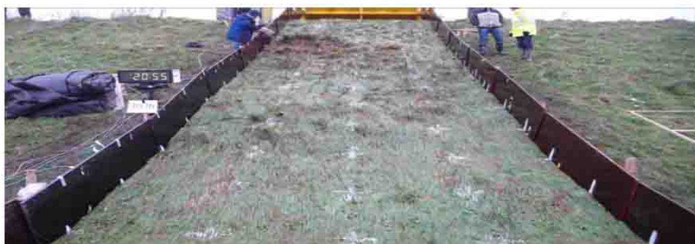
FIGURE 8.5: Tielrode overtopping experiment result test section 2. Picture from the factual report published by Flanders Hydraulics Research [22]
