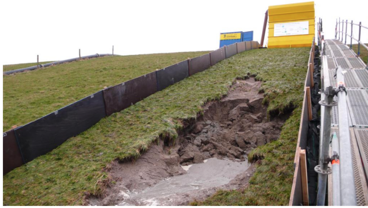
FIGURE F.4: Final result of the fourth Frieze Waddenzeedijk overtopping experiments. Photo taken by Infram B.V. [3]
