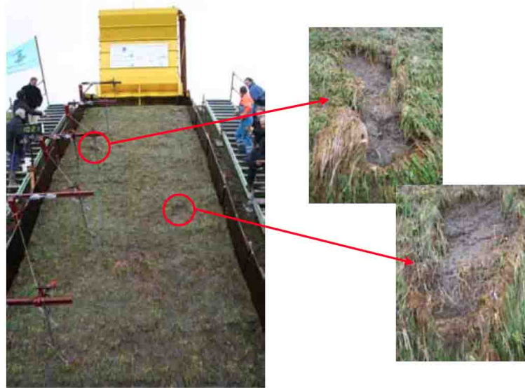
FIGURE 8.11: Initial damage spots during the St Philipsland overtopping experiments. Photo taken by Infram B.V. [4]
