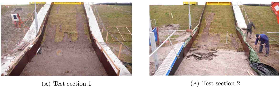
FIGURE 8.8: Final result of the wave overtopping experiments at the Afsluitdijk, February 2009. Photo's taken by Infram B.V. [5]
