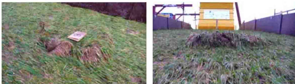
FIGURE F.7: Initial damage spots noticed during the second Kattendijke overtopping experiments. Photo taken by Infram B.V. [4]
