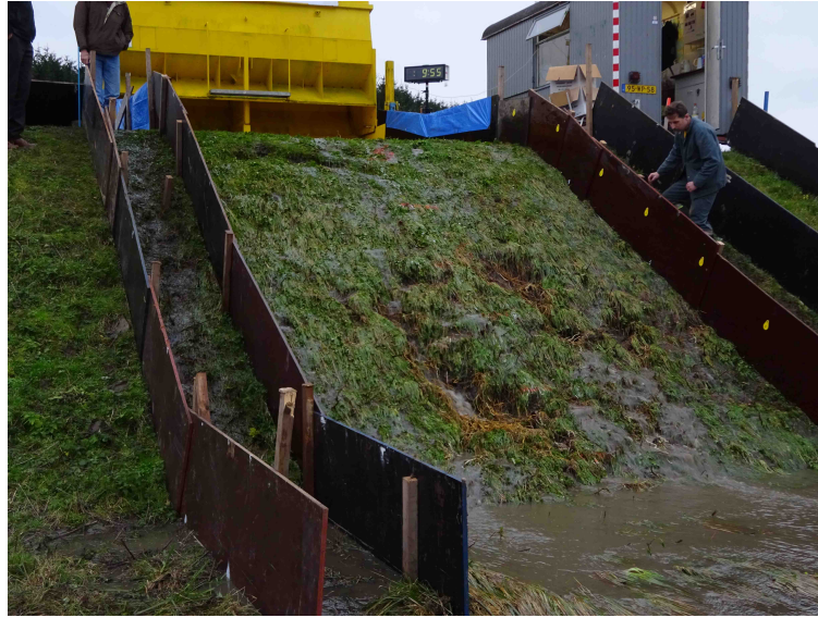
FIGURE 8.2: Initial damage during the second overtopping experiments occurred in grid section 7.
