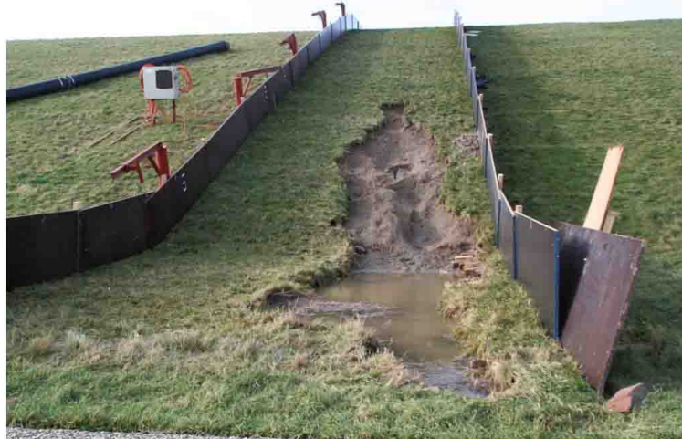
FIGURE F.3: Final result of the third Friese Waddenzeedijk overtopping experiments. Photo taken by Infram B.V. [3]
