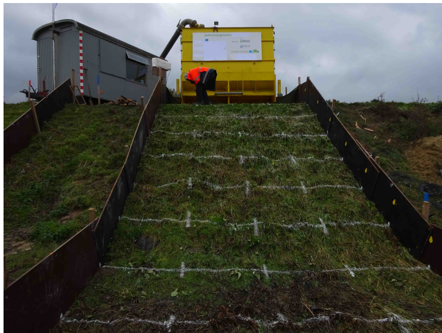
FIGURE 3.6: Test section for the first overtopping experiment.
