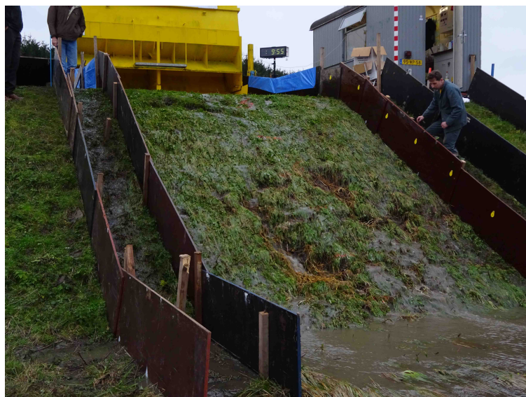
FIGURE F.1: Initial damage during the second overtopping experiments occurred in grid section 7.
