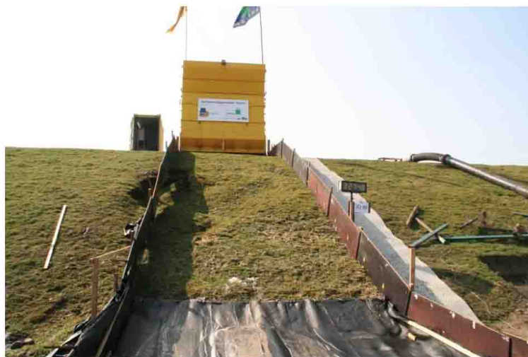
FIGURE F.9: Final result second overtopping experiment Tholen, the land side slope collapsed completely due to the washing away of the sand core by groundwater flow. Photo taken by Infram B.V. [6]
