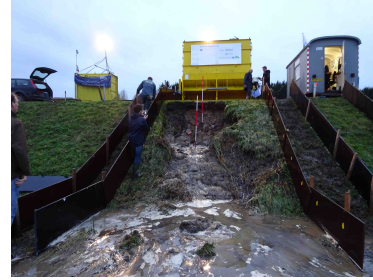
(B) Final result overtopping experiment 2.
