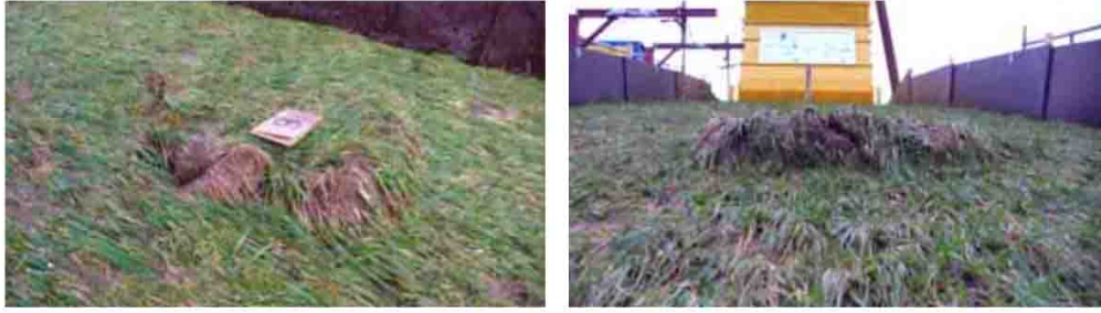
FIGURE 8.14: Initial damage spots noticed during the second Kattendijke overtopping experiments. Photo taken by Infram B.V. [4]
