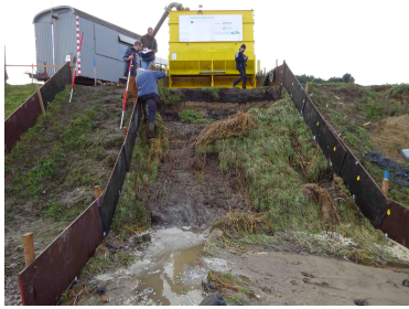
(A) Final result overtopping experiment 1.
