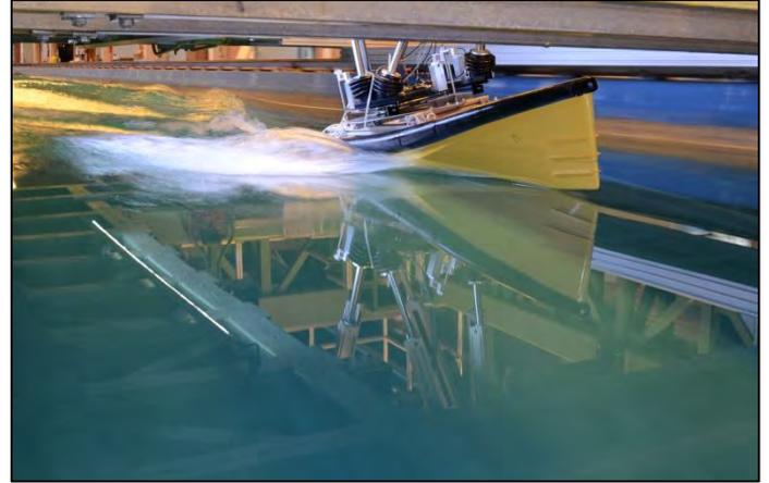
Figure 3 Model test run (Stage 1,  $Fr = 1.05$ ,  $\phi = 12$  deg)
