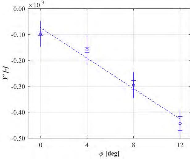
Figure 4 Sway force due to heel (Stage 1, Fr = 1.05)
