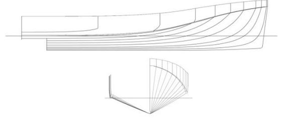
Figure 2 NH 1816 hull lines
