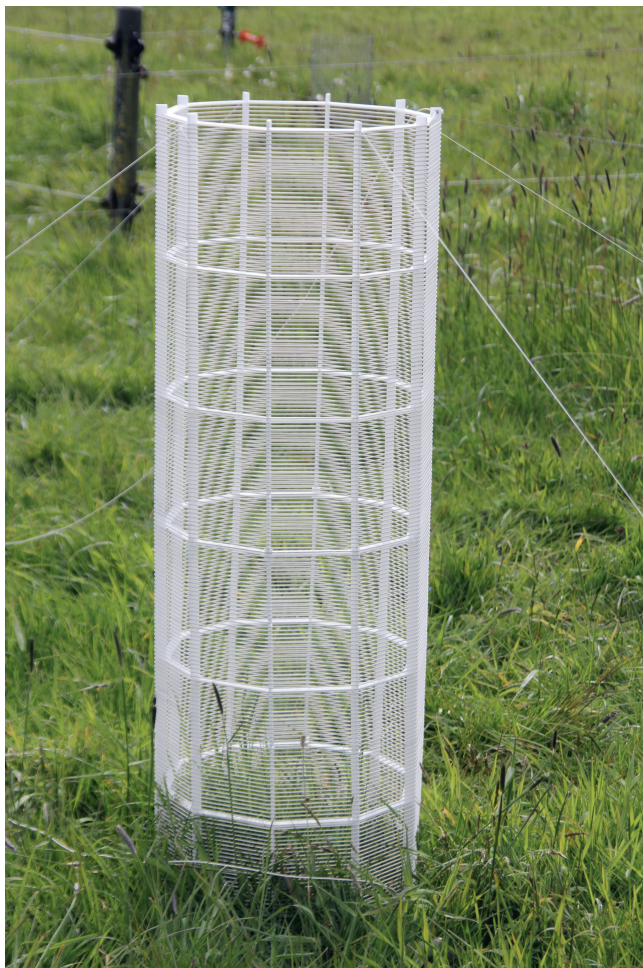
Figure 6.3: DTS coil to measure near-surface air temperatures above and inside the grass layer. Photo by Tijn ter Horst.
