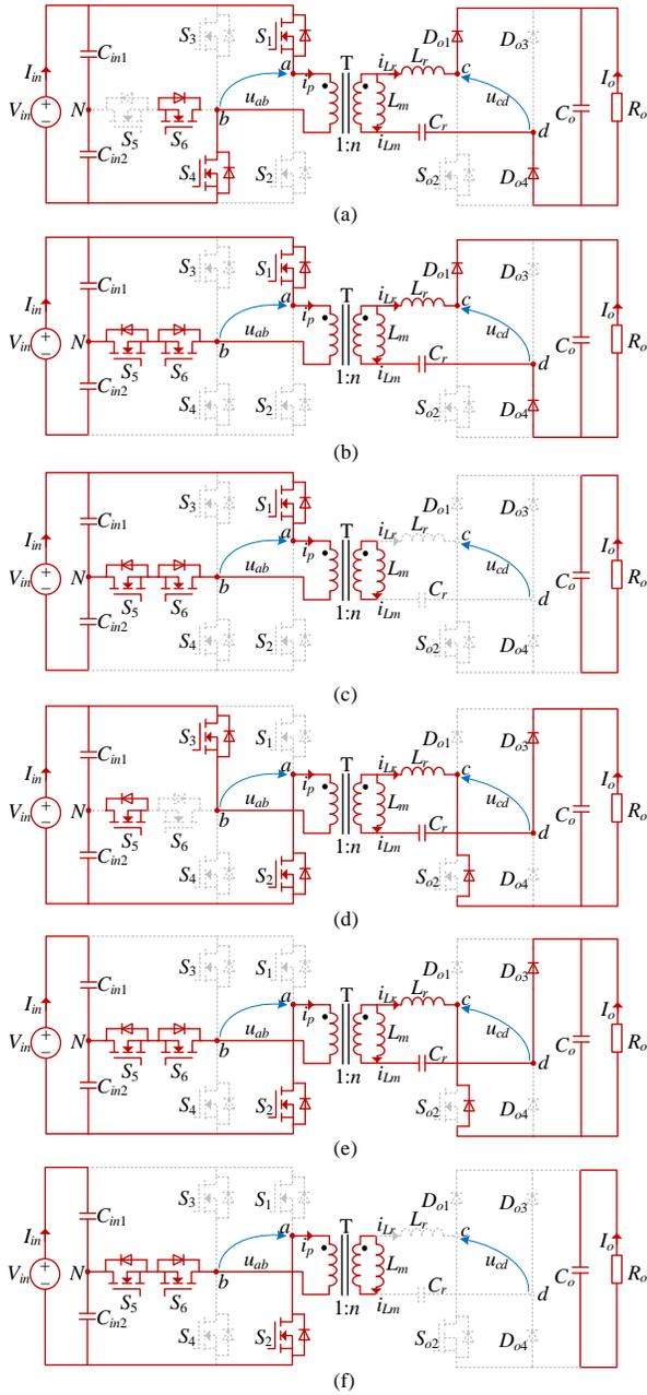
Fig. 5. Equivalent circuit of each switching state in the LV output mode: (a) Stage I  $[0, \phi]$ ; (b) stage II  $[\phi, \alpha]$ ; (c) stage III  $[\alpha, \pi]$ ; (d) stage IV  $[\pi, \pi+\phi]$ ; (e) stage V  $[\pi+\phi, \pi+\alpha]$ ; (f) stage VI  $[\pi+\alpha, 2\pi]$ .
