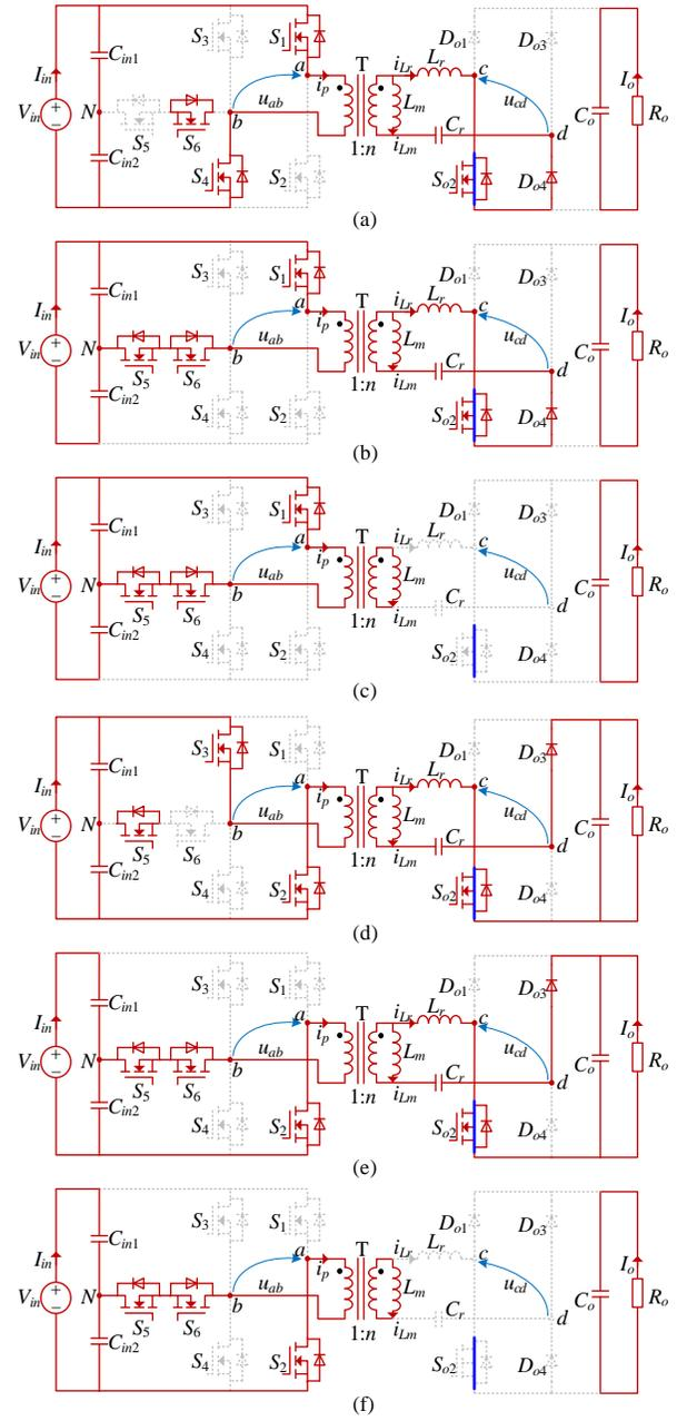
Fig. 6. Equivalent circuit of each switching state in the HV output mode: (a) Stage I  $[0, \phi]$ ; (b) stage II  $[\phi, \alpha]$ ; (c) stage III  $[\alpha, \pi]$ ; (d) stage IV  $[\pi, \pi+\phi]$ ; (e) stage V  $[\pi+\phi, \pi+\alpha]$ ; (f) stage VI  $[\pi+\alpha, 2\pi]$ ;
