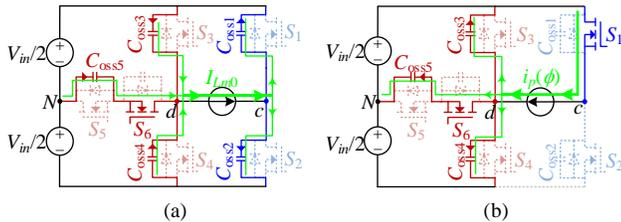
Fig. 10. ZVS mechanism of primary-side switches. (a) ZVS-on of  $S_1$  and  $S_4$  at  $t = 0$  (see Fig. 4), (b) ZVS-on of  $S_5$  at  $t = \phi / \omega$ , (i.e.,  $\theta = \phi$ , see Fig. 4).
