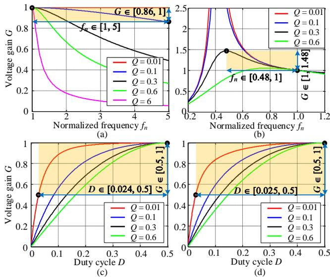
Fig. 12. Voltage gain characteristics of the conventional full-bridge SRC and LLC resonant converter. (a) SRC with PFM control; (b) LLC resonant converter with PFM control; (c) SRC with PWM or PSM control; (d) LLC resonant converter with PWM or PSM control.
