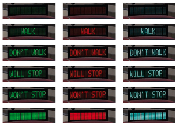
Fig. 2. Cropped screenshots of the videos, showing the eHMIs used in this study for the roof position (5 messages + 1 ‘no activation’) x 3 colours.
