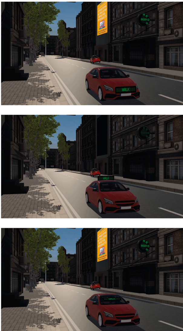
Fig. 3. Screenshots of the videos, showing eHMI with the green message 'WALK' placed on the front bumper (top figure), the roof (middle figure), and the windshield (bottom figure). Distractions are on in the top and bottom figures; distractions are off in the middle figure.
