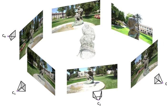
**Figure 2-8:** Collection of input images with known poses  $\mathcal{T}$  and sparse 3D point cloud model  $\mathcal{X}_s$ . The data set was obtained from the Ignatius data set of the Tanks-and-Temples benchmark [36].
