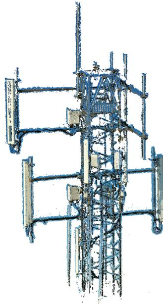
**Figure 3-4:** The reconstructed dense 3D point cloud model of COLMAP after increasing the number of features. Note that PIX4D failed to compute a reconstruction.
