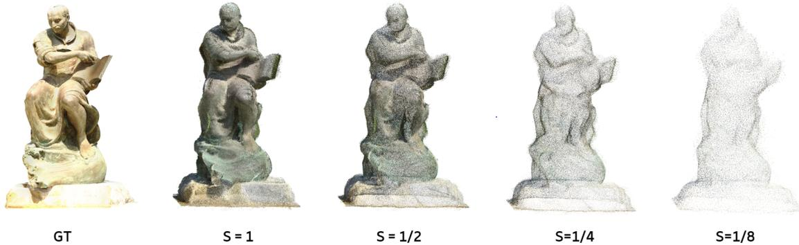
**Figure 5-3:** Dense 3D point cloud reconstructions at different downscale factors  $S$  compared against the ground-truth (GT).
