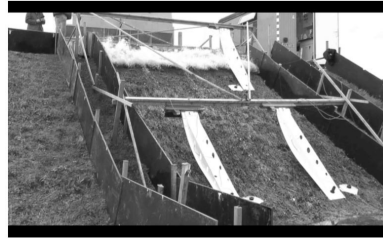
(a) Overtopping at the crest
