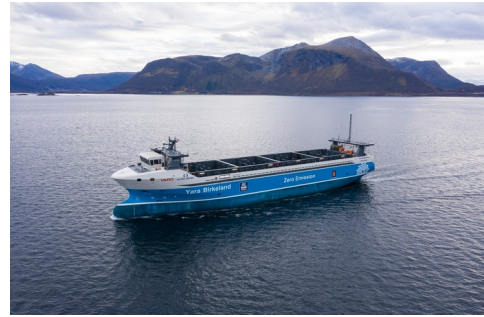
Figure 1.2: Yara Birkeland is the world's first fully electric and autonomous container vessel with zero emissions. With this container vessel, Yara will reduce diesel-powered truck haulage by 40,000 journeys (approximately 1,000 tonnes of CO 2 ) a year. [5]
