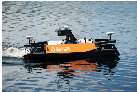
Figure 1.4: The "Otter" USV by Maritime Robotics is designed for hydrographic surveying and bathymetric mapping, offering a cost-effective, portable solution for precise data collection in sheltered and shallow waters. [8]
