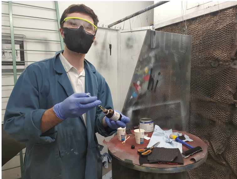
Preparing the polyurethane glue solution with activator
