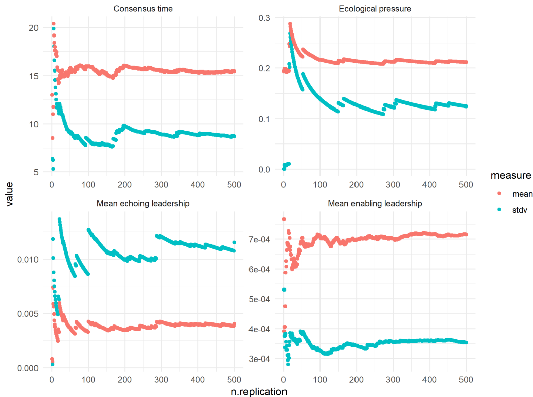
Figure 5.9: Cumulative mean and standard deviation of KPIs for 500 replications of one of the initial scenarios analyzed (population of 40 and density of 0.2)
