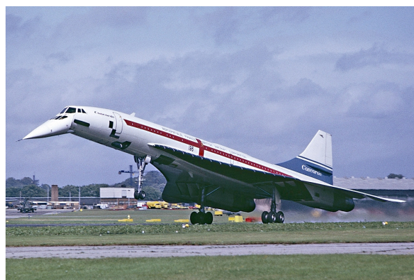
Figure 1.4: The Aérospatiale/BAC Concorde with its droop nose lowered to provide the pilots a higher overnose angle 6
