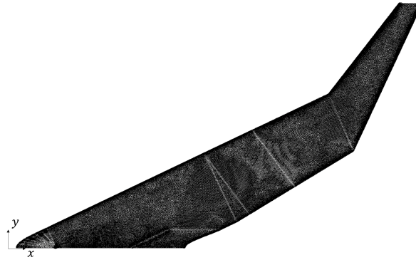
Figure 4.1: A mesh generated for the Flying V with integrated cockpit and center fairing using a low element count
