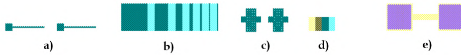
Figure 4.13: a) Release test b) Aspect ratios c) Etch hole test d) CNT growth test e) Contact pad test
