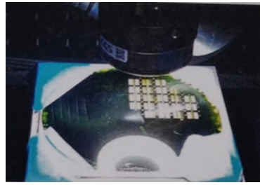
(a) The femto-second laser setup with a 4H-SiC wafer on the chuck [6]
