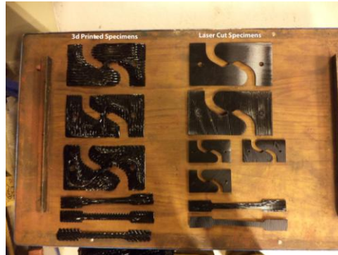
Figure 4: Left: the specimens that are directly printed within the xy-plane. Right: Specimens that are laser-cut from plates that are printed within the xz-plane.
