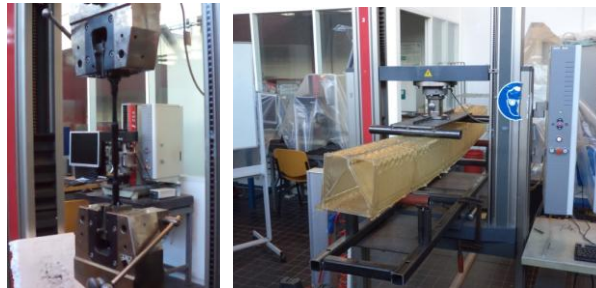
Figure 5: Left: One of the Elementary test-setups, the performance of a Tensile test. Right: One of the tests on Block/Geometry level: the bending test of a square tube beam with an inner triangular structure.
