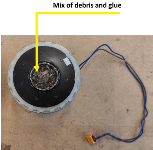
(D) Clogged Motor From Vacuum Cleaner With Mix Of Debris And Glue
