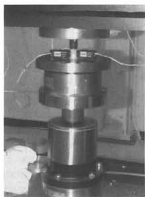
Figure 3. Photograph of the Young's Modulus test setup and results of a 500 pound load run.
