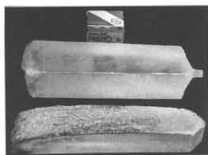
Figure 3. CsI(Tl) crystals obtained by VB method (upper) and HB method (lower) with length about 25cm
