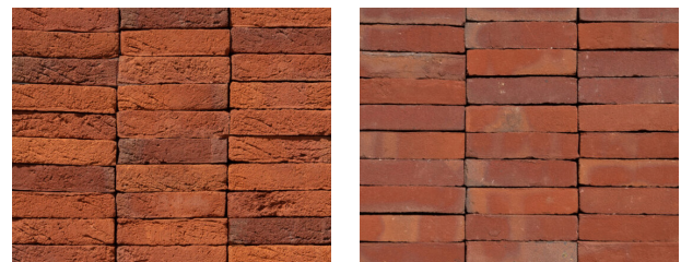
Fig 31. hand-moulded brick (left) and (machine-)moulded brick (right), (Vogelensangh).
