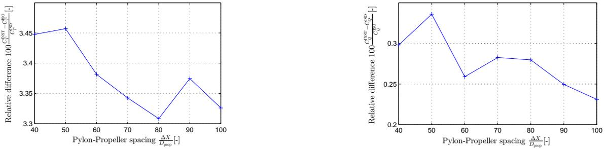
**(a)** Installation effect on Thrust Coefficient
