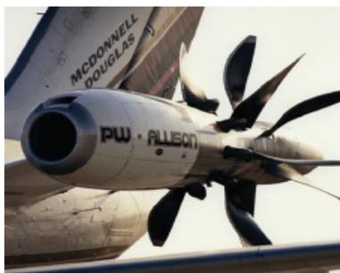
**Figure 1.2:** PW/Allison 578 DX on MD-80 aircraft [7]
