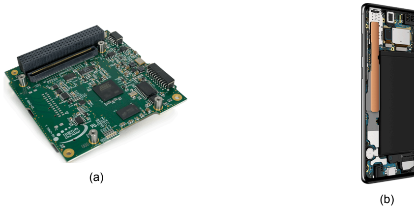
Figure 4.4: In 4.4a a modern on board computer for a CubeSat spacecraft from [21]. In 4.4b the motherboard of a modern smartphone from [40]. Certainly size and form of the components is similar.
