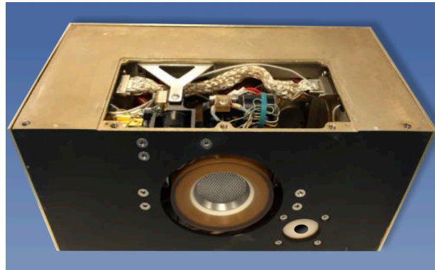
Figure 7.1: BIT-3 engine module [90] used in the Lunar IceCube mission [28], representative of the acceleration level considered.
