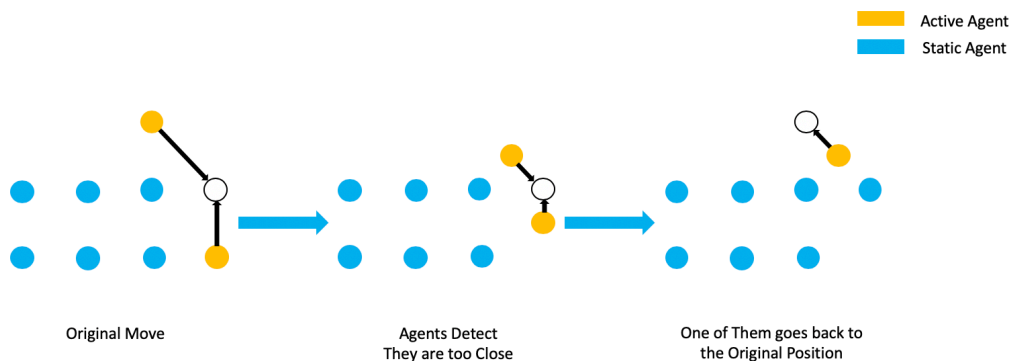
Figure 7.2: Collision avoidance strategy. Both active agents target the same position. They move towards it, but when they detect they are too close, one of them goes back to its original position whilst the other one finishes the maneuver.
