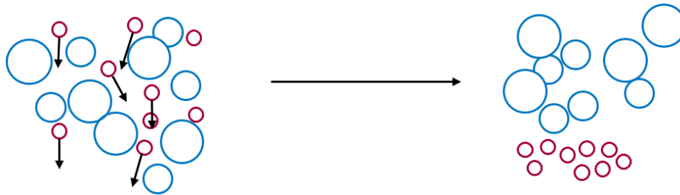
Figure 2.4: Segregation by percolation.
