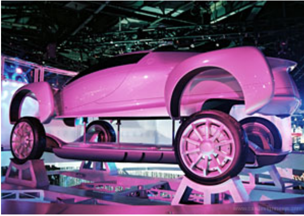
Figure 28: The chassis and skateboard of the skateboard car (source: www.gm.com )
