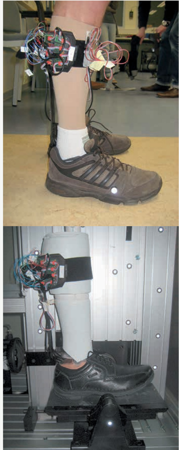
Figure 36. Top: Orthosis with integrated strain gauges on a patient in order to measure loads on AFO during real life gait. Bottom: Same orthosis with integrated strain gauges on a dummy leg in a load cycle test setup to verify if the applied loads are correct (Hochmann, 2014).
