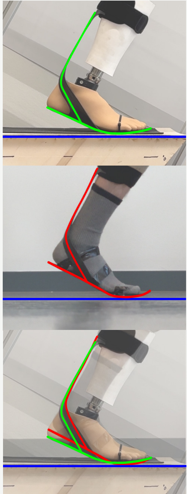
Figure 65. Testing forefoot rocker . The top image is the test setup, the middle is the reference video, and the bottom is the comparison.
