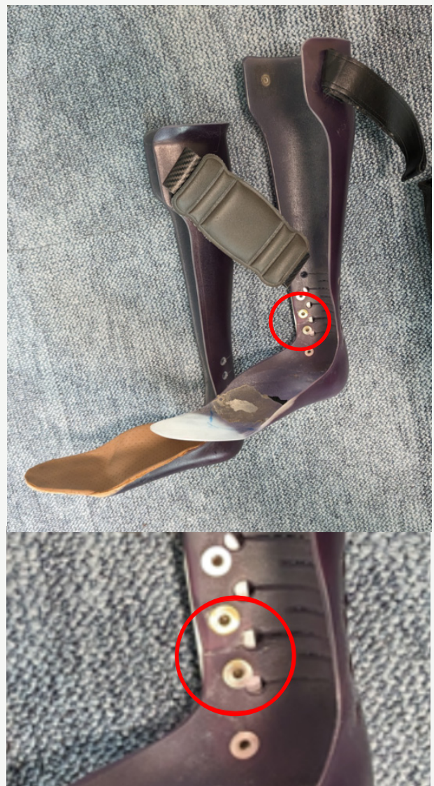
Figure 17. Failed PP AFO, repaired with a metal strip.
