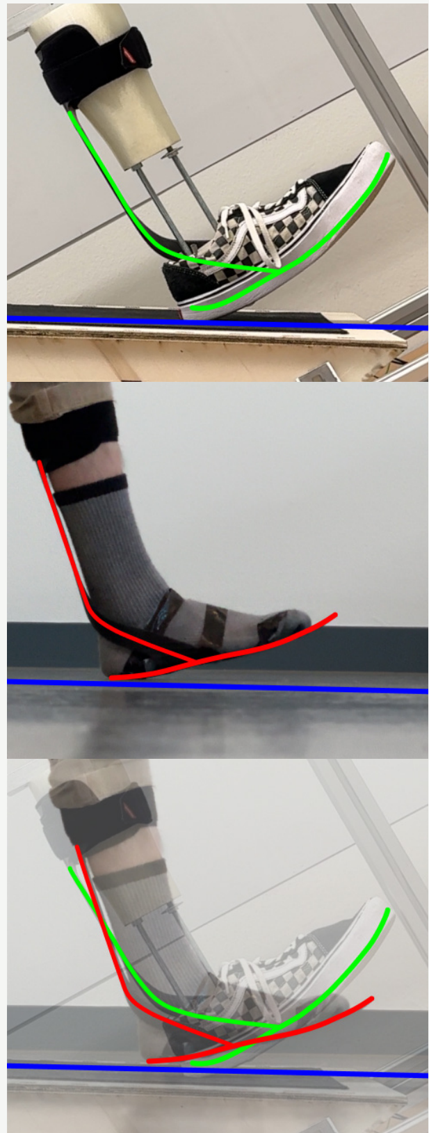
Figure 41. Testing heel rocker with the realized test setup (top image) and comparing it to the reference video (middle and bottom image).
