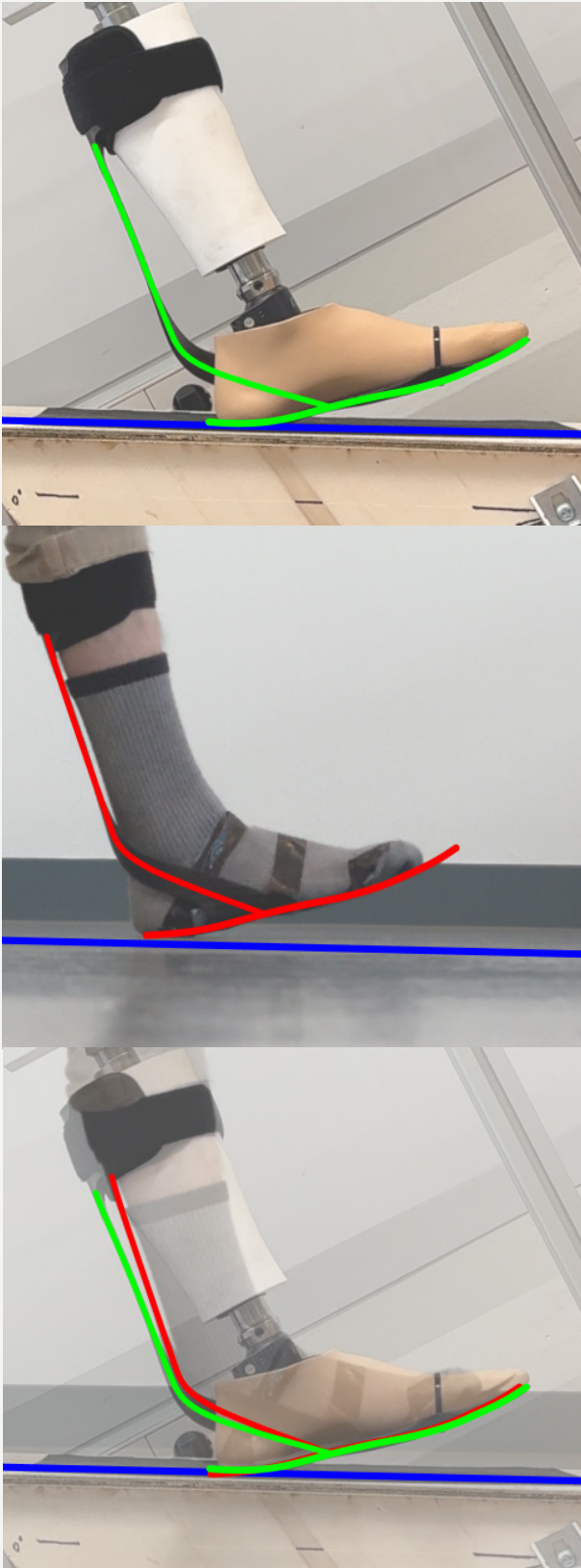
Figure 64. Testing heel rocker . The top image is the test setup, the middle is the reference video, and the bottom is the comparison.
