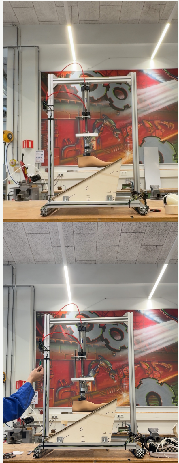
Figure 61. Top before with the original leaf spring, bottom after replacing the leaf spring with the PP and aluminium plate combination. See how, in the bottom image, the foot bends around the toes.
