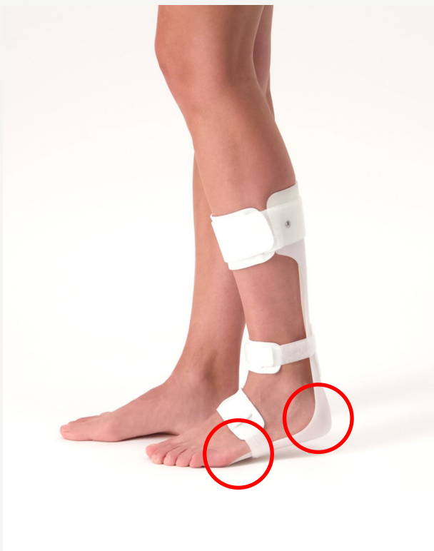
Figure 16. Failure hotspots in PP AFOs, some wear around the MTP and but mainly around these two spots in the neck area of the AFO.
