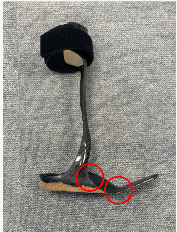
Figure 15. In this picture a carbon AFO made through wet lamination is shown, as no broken carbon prepreg AFOs was at hand. The failure hotspots, however, are the same in carbon prepreg AFOs, 50% around the MTP and 50% around the neck area of the AFO.
