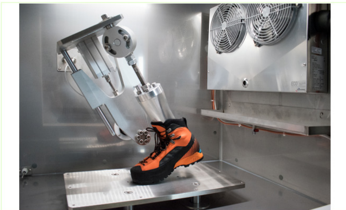
image / figure 2 A possible to be developed test setup: a load cycling machine (example ski boot tester by STEP lab).
