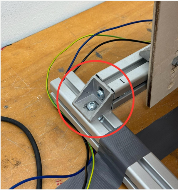
Figure 49. The bolts of the frame came loose due to the vibration of cycling.
