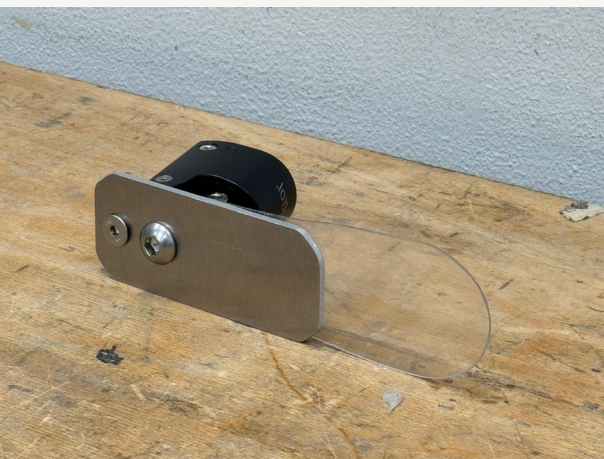
Figure 60. The solution: combination of a super flexible full-foot PP plate with a stiff aluminium plate running until the point where the MTP joints are located. This way, the toes of the foot will be able to bend.
