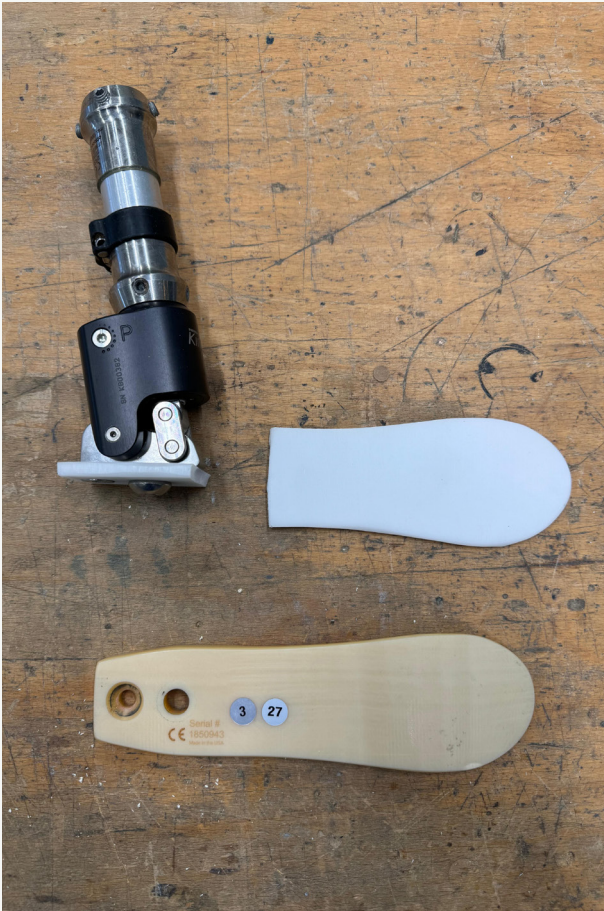
Figure 59. The original leaf spring making within the foot part of the prosthetic was too stiff, so it was tried to replace it with a more flexible polymer. The polymer, however, could not provide the necessary bending and broke.
