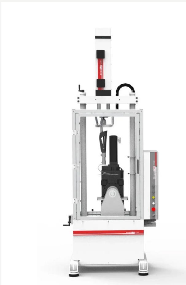
Figure 27. ISO 22675 based load cycle test equipment for prostheses made by STEP Lab (2024).
