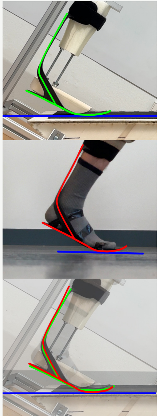
Figure 43. Testing heel rocker with the realized test setup and comparing it to the reference video. Top is the test setup, middle the reference and bottom the comparison.
