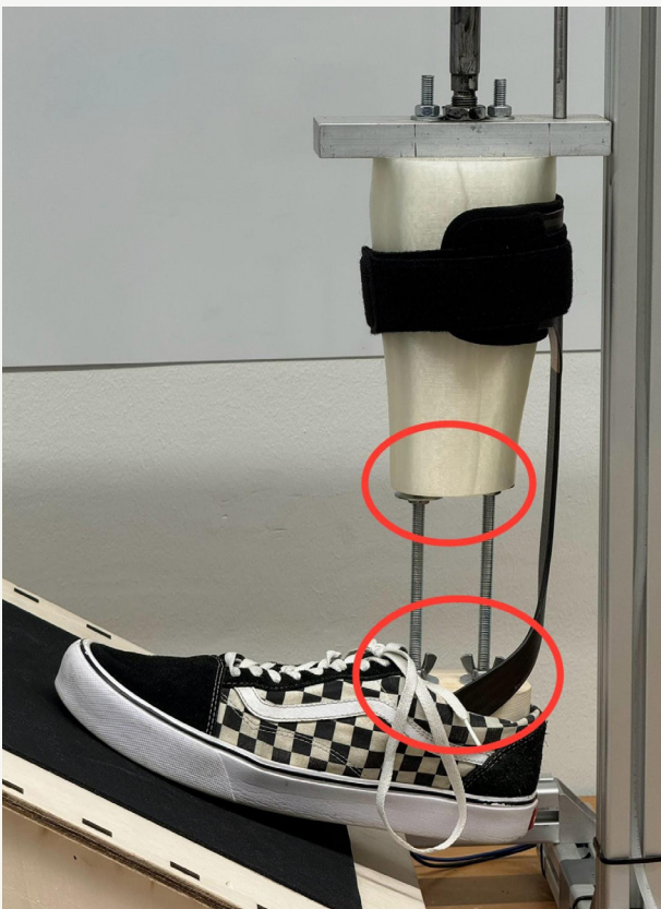
Figure 50. The bolts of the dummy leg came loose due to vibration of cycling. The lower ones are hand tightened. Thread-locker and nuts could fix this.
