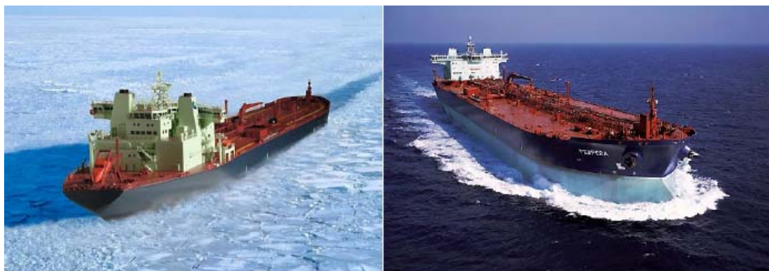
Figure 4.6 Tempera Double Acting Tanker travelling astern to break the ice and, to the fore proving its efficiency in open water (Source: Shi, 2009)
