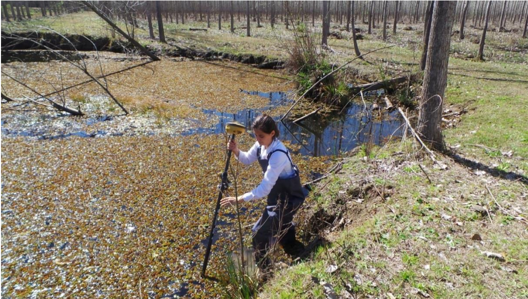
FIGURE 16 MEASUREMENT OF RIVER PROFILE AFTER A DYKE BREACH
