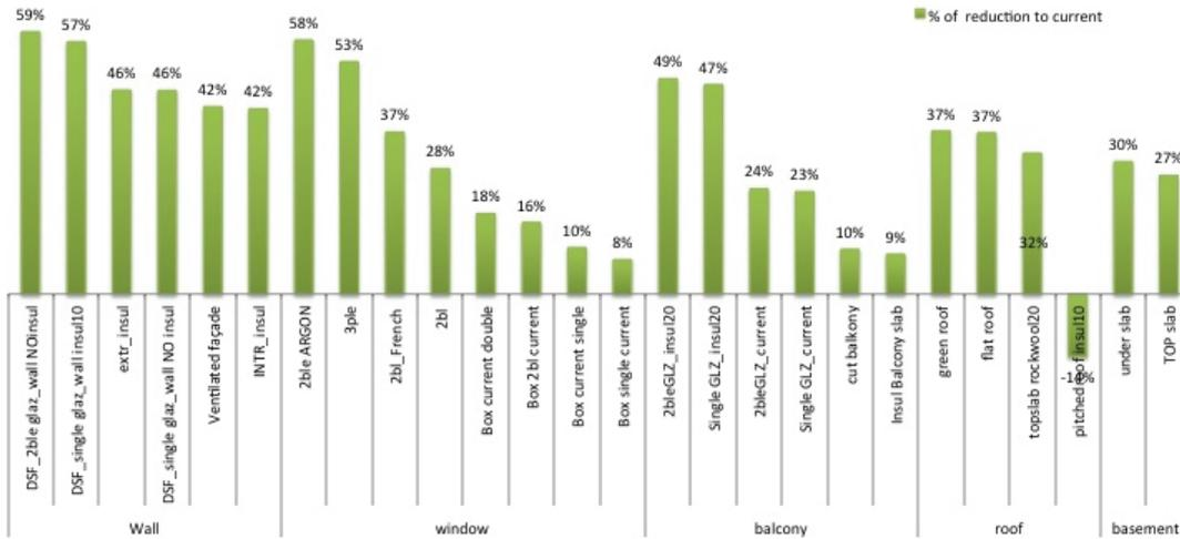
Fig.1. Quantification of the energy demand reduction by the implementation of the individual measures
