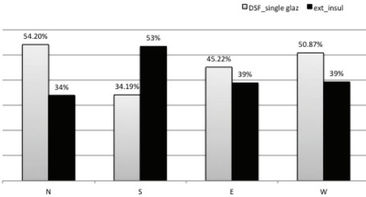
Fig.2. The reduction (%) to current heating energy demand after the implementation of a second skin glazed façade and external insulation, according to different orientation.
