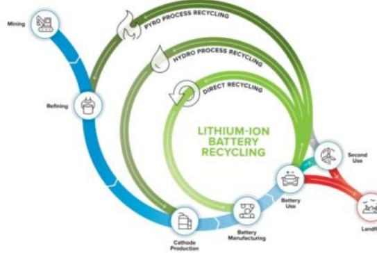
Fig. 2 The recycling routes for materials in batteries each process returns the materials to another step in the manufacturing process. Source: ReCell Center
