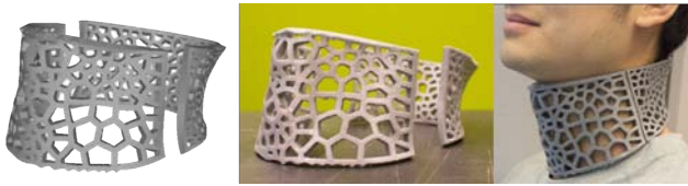
Figure 10. Optimized neck cast in two pieces. (Left) Digital model, and (right) 3D printed neck cast worn by the user.
