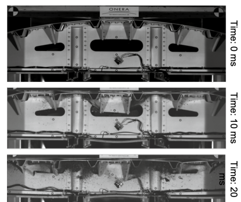
Figure 7.5: Crash results of a composite fuselage section [16].
