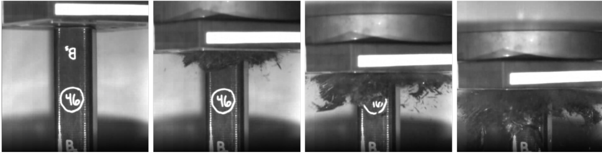
Figure 4.3: Square tube crush specimen test results pictures.
