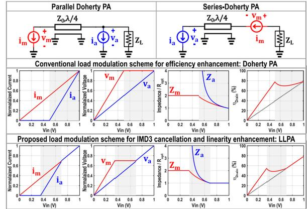
Fig. 3. Parallel and series DPAs' simplified structures (top), the load modulation scheme of conventional DPA (middle), and the proposed load modulation scheme for IMD3 cancellation (bottom).
