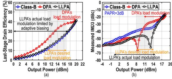
Fig. 5. (a) CW and (b) two-tone IMD3 measurement results versus output power.
