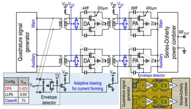
Fig. 4. Schematic and die photo of the employed 28 GHz series-DPA to realize the proposed LLPA.
