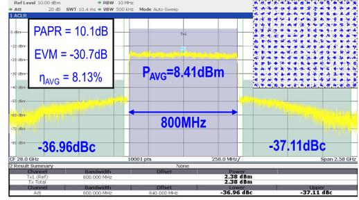
Fig. 7. Measured spectrum and constellation of an 800 MHz 256-QAM OFDM signal.
