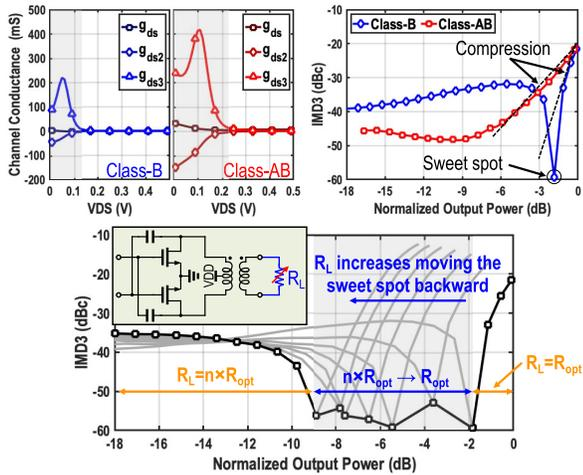
Fig. 2.  $g_{ds}$ ,  $g_{ds2}$ , and  $g_{ds3}$  versus VDS and the two-tone simulation results of class-B and class-AB PAs (top). The two-tone simulations for various  $R_L$  exhibiting IMD3 sweet spot at lower output power levels (bottom).
