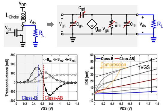
Fig. 1. Equivalent model of a common-source PA. The simulated  $g_m$ ,  $g_{m2}$ , and  $g_{m3}$  of a 40 nm nMOS transistor versus gate bias voltage and drain-source current versus drain-source voltage are given.
