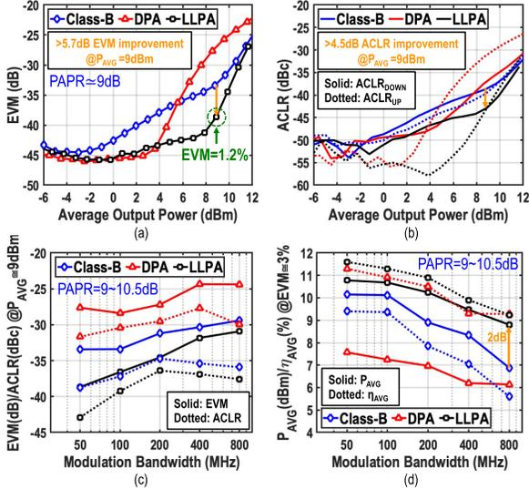
Fig. 6. Measured (a) EVM and (b)  $ACLR_{DOWN}$  (solid)/ $ACLR_{UP}$  (dotted) of a 50 MHz 64-QAM OFDM versus  $P_{AVG}$ . (c) Measured EVM (solid) and ACLR (dotted) for the 64-QAM OFDM signals at 9 dBm  $P_{AVG}$ . (d)  $P_{AVG}$  (solid) and  $\eta_{AVG}$  (dotted) when EVM = 3% for 64-QAM OFDM signals.
