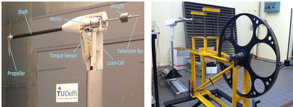
(a) Photograph of the Propulsor with Semi-Casing (b) Propulsor Integrated Load Cell Calibration Setup
