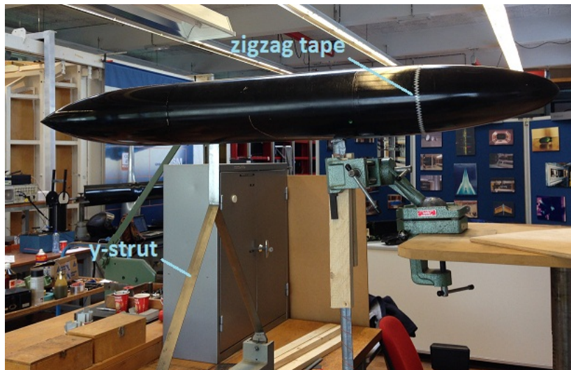
Figure 6-4: Photograph of the Body with Struts in Vibration Test Configuration
