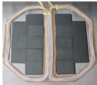
Figure 3-VIII Double D coils FEM Simulation Model and Double D coil photo
