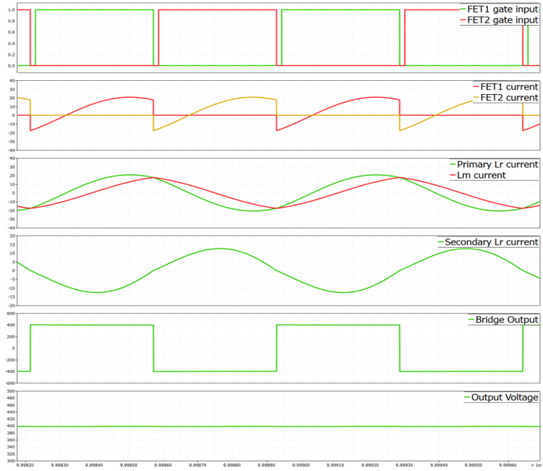
Figure 4-XVI Operation at the primary resonant frequency - Waveforms
