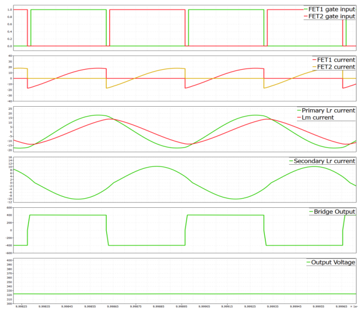
Figure 4-XVIII Operation above the primary resonant frequency - Waveforms
