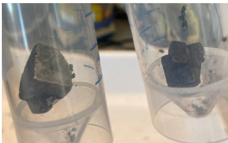
Figure A-8 Cubic Pyrite seeding crystals recovered at the end of the experiments inside the anoxic glovebox. Clear black deposits visible.
