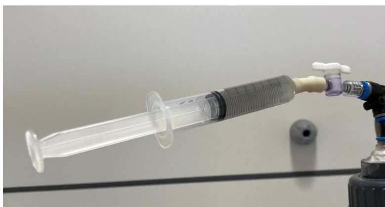
Figure A-5 Effluent sampling via syringe showing clear blackening of the solution. Samples taken during dosing ratio \text{Fe}:\text{S}^{2-} = 1:2
