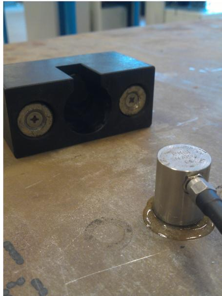
Figure 6.5: A view on the location where the signal strength was measured. The sensor is connected to the metal plate using acoustic couplant gel, and the black block is used to apply a constant force on the sensor, by making use of two magnets which are attached to springs.
