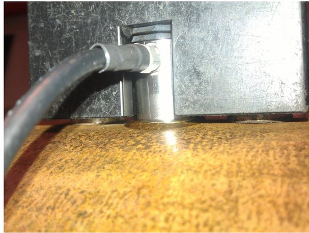
Figure 6.8: The test setup at the smaller tube with rusted surface. The sensor is held in place using magnetic hold downs, and acoustic couplant gel is used to maximize transmission of signal between the surface and the sensor. The surface has been cleaned using water and dry cloth to remove any dust or debris, but rust is not removed.
