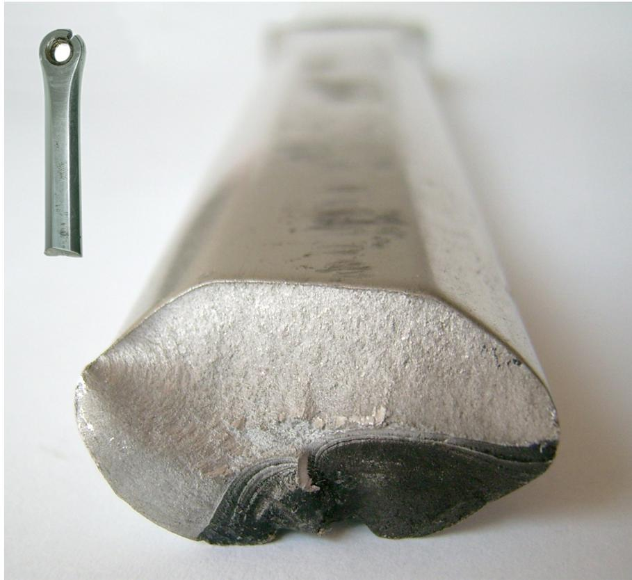
Figure 3.1: An example of a bicycle crank that has failed due to fatigue. The crack started to grow in the black area, until at some point the remaining cross sectional area (light/silver) failed. Note that the lines in the crank indicate the size of the crack growth, and the lines have a larger distance in-between as the crack increased in size. [35]
