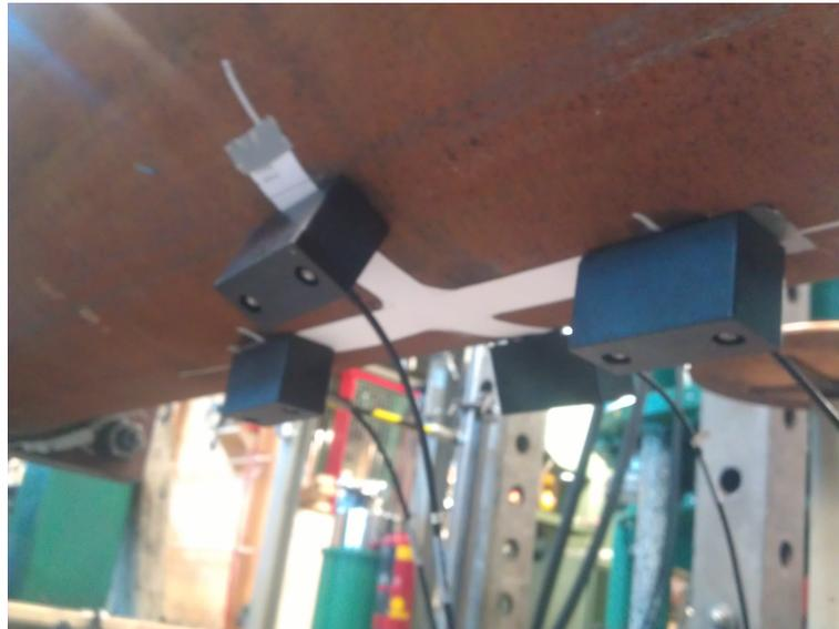
Figure 6.14: Sensors applied to the structure; the template has not been removed, as the holes cut into the template allow for maximum transmission.
