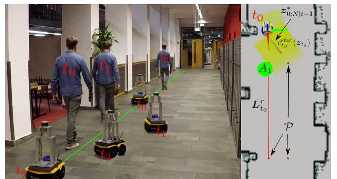
Fig. 17: Avoiding an oncoming pedestrian in a corridor. (left) real-world experiment (right) online visualization.
