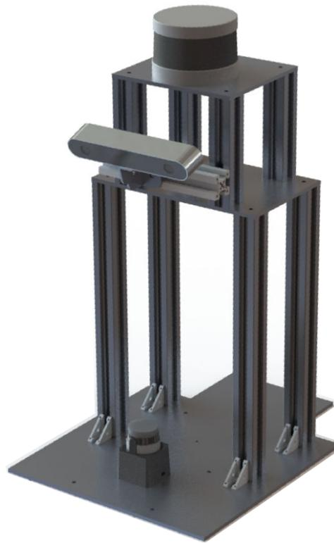
**Figure C-4:** CAD drawing of the designed sensor mount
