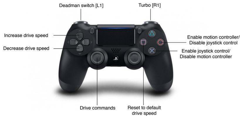
**Figure C-6:** Joystick controls layout.
