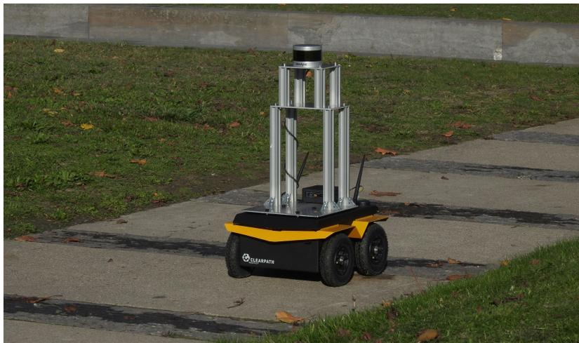
**Figure C-1:** Jackal robotics platform, designed by Clearpath™ Robotics.
