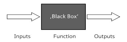
Figure. 7: "Blackbox" system model by Eekels and Cross for a function (Klein, 2013)
