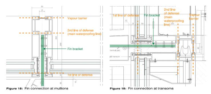
Figure. 46: Panel watertight barriers and connections wit horizontal and vertical fins. Drwaings provided by Eckersley O'Callaghan
