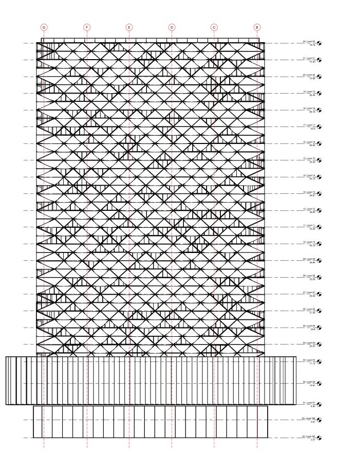
Figure. 116: West facade with proposed shading system
