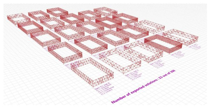
Figure. 95: Export of 23 solutions out of the 300 generated. Out of these solutions 4 of them 4 are the extreme solutions, meaning the fittest for each one of the four objectives and the rest are the last generation solutions. They are 23 in total and not 24 because individual id0 of the G14 (14th generation) happens to also be the fittest in terms of fitness objective 4 which in this case is the one with the minimum, maximum displacement.
