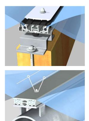
Figure. 20: Typical details for ETFE steel and wooden support frame structures, cushion frames, cushion panels as well as inflation system installation
