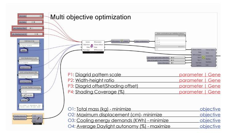
Figure. 90: Walacei workflow, input parameters, objectives and geometries to be generated
