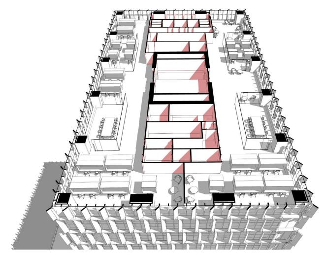
Figure. 39: The core and the perimeter functions of the tower.
