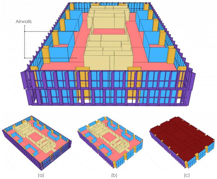
Figure. 62: Final energy model preview a. with original unitized panels and fins, b. with simplified fins and c. with top and bottom floor of the segment to be investigated.
