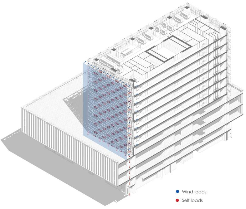
Figure. 110: Vertical and horizontal load transfer
