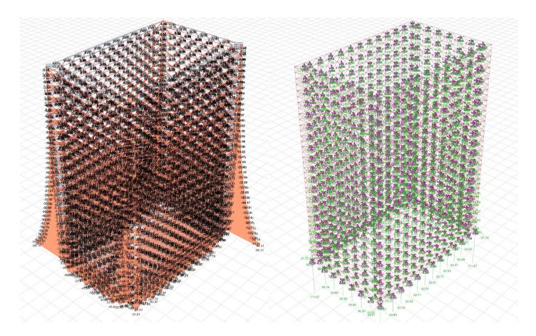
Figure. 101: Static analysis for the whole bearing structure of the shading system
