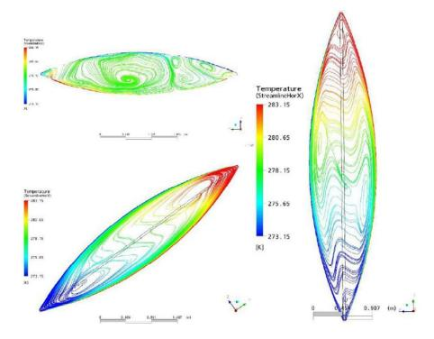
Figure. 17b: One-chamber-cushion different assembly situations and air flow inside the cushion panels with temperatures Ti=20°C (inside) and To=-10°C (outside) (Kersken et al., 2021)
