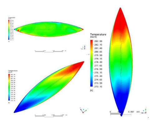
Figure. 17a: One-chamber-cushion different assembly situations and heat flow directions with temperatures Ti=20°C (inside) and To=-10°C (outside), (Kersken et al., 2021)
