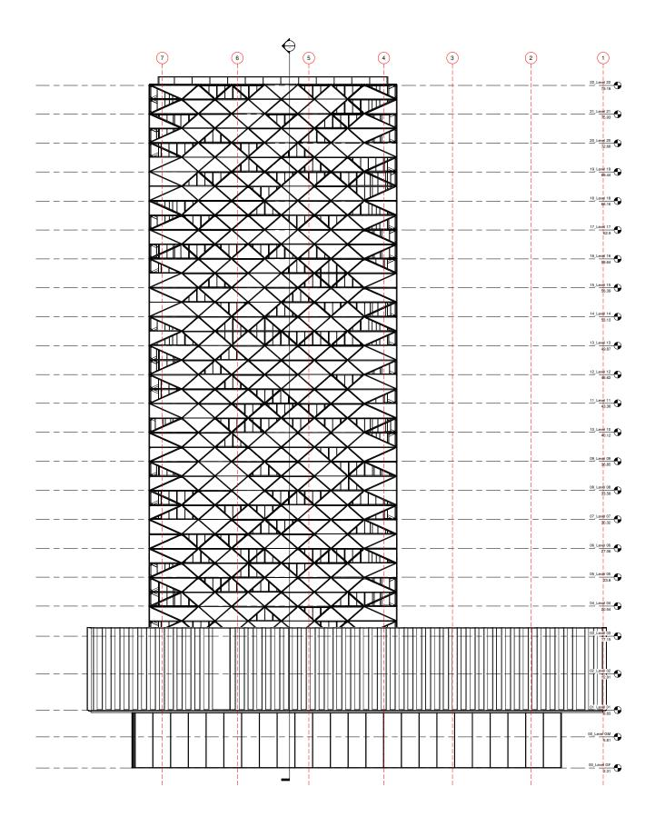
Figure. 117: North facade with proposed shading system
