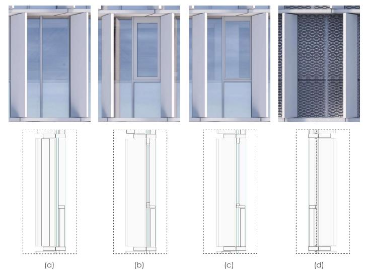
Figure. 41: The tower's different panel types, a. Panel with fixed glazing, b. Panel with operable window, c. Panel with fixed window, d. Metal mesh MEP panel, drawings provided by Eckersley O'Callaghan
