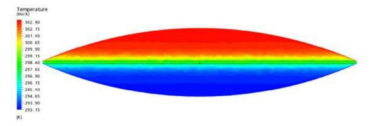
Figure. 18: One-chamber-cushion vertical heat flow (downward) with temperatures Ti=20°C (inside) and To=30°C (outside), (Kersken et al., 2021)
