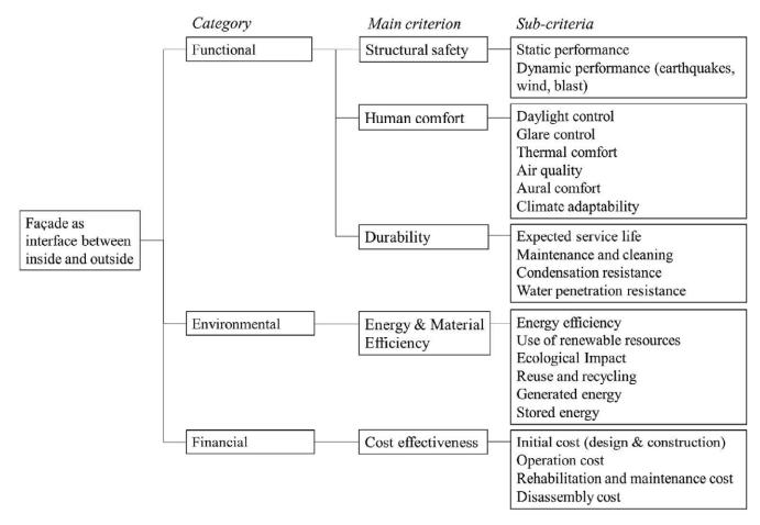
Figure. 10: Another approach to the facade function tree (Bianchi et al., 2024b)
