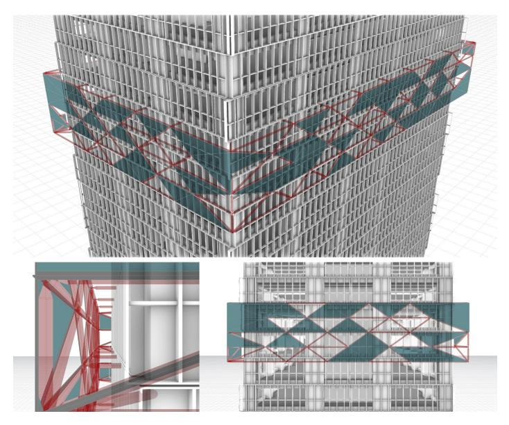
Figure. 82: Shading system approach with self standing bearing structure
