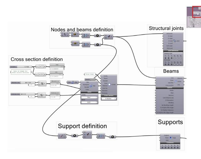
Figure. 83: Translating the already defined geometry of the shading system into Karamba Beams, Supports and Joints. Source for EN 10210 cross section: (http://www.b2bmetal.eu/en/pages/index/id/105/)
