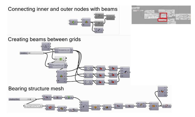
Figure. 78: Definition of diagrid patterns and of the in-between beams based on slab heights
