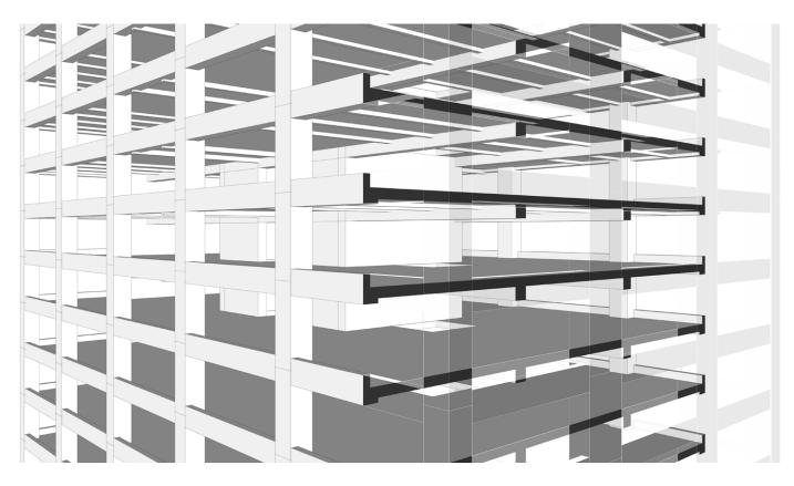
Figure. 38: Piraeus Tower main bearing structure out of reinforced concrete. Drawing by Alkiviadis Oikonomidis based on provided drawings by Eckersley O'Callaghan
