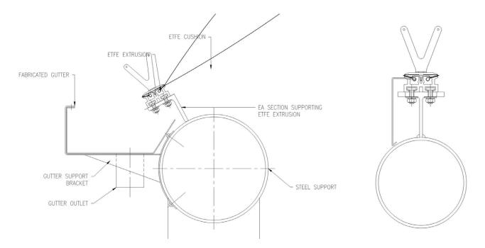
Figure. 19: Typical details for ETFE steel support frame structures, cushion frames and cushion panels
