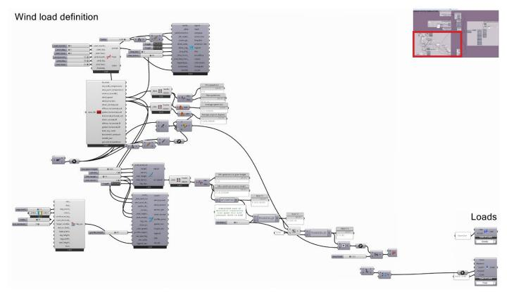
Figure. 84: Extraction of wind direction and speed and translation of wind speed into wind pressure
