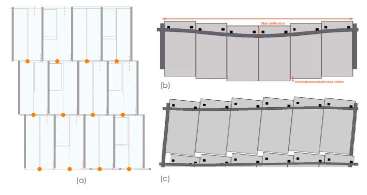
Figure. 43: Panel a. stopper elements and movements due to local deformations, b. creep and c. interstorey drift Drawings provided by Eckersley O'Callaghan
