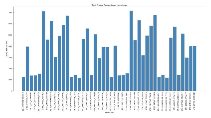
Figure. 70: Total cooling demands for each room/zone in the typical floors under investigation
