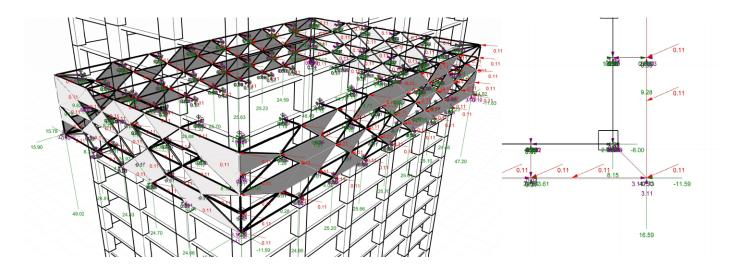
Figure. 86: Translation of shape into a static model, application of loads, supports and reactions calculation
