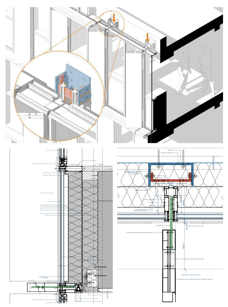
Figure. 42: The panels structural details. Movement accomodation at the top, typical details and connection with horixontal and vertical fins at the bottom. Drawings by Alkiviadis Oikonomidis based on provided drawings by Eckersley O'Callaghan
