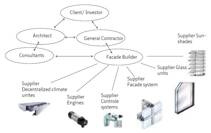
Figure. 5: Scheme of the relationship between different roles in façade design (Klein, 2013)
