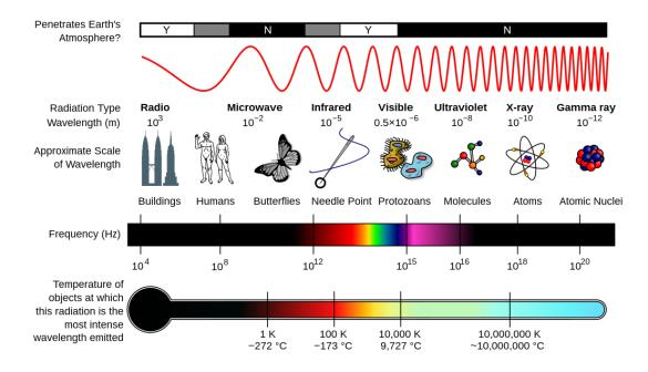
Figure. 16: Electromagnetic spectrum (wikipedia)
