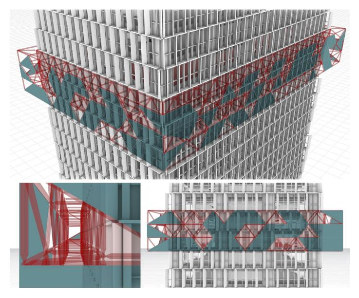
Figure. 76: Shading system approach with self standing bearing structure
