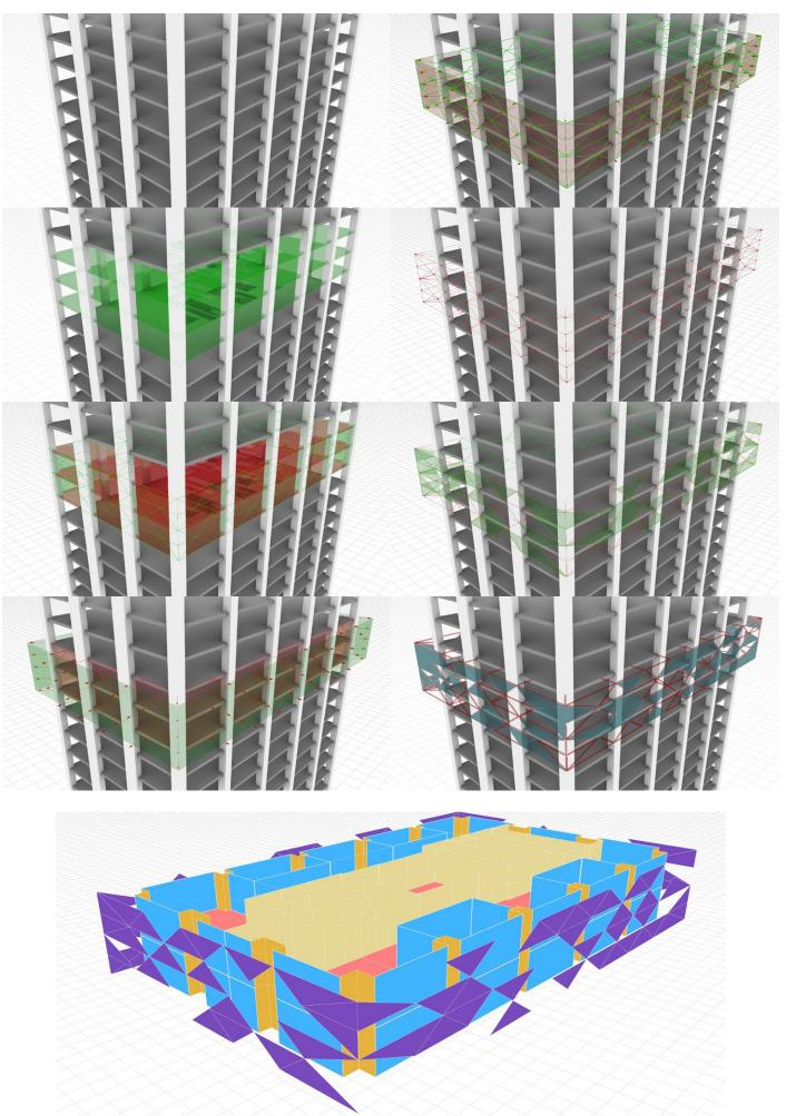
Figure. 80: Consecutive steps for defining the exoskeleton shading system in relation to the tower 's main bearing structure and the end resault energy model
