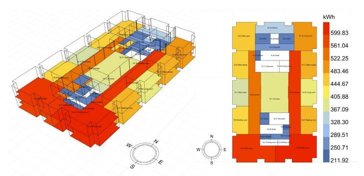
Figure. 99: Total zone Ideal Loads supply air Total cooling energy 3 Aug to 9 Aug from 0.00 to 23.00
