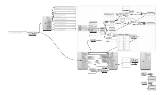
Figure. 33: Ladybug-Dragonfly workflow to affect EPW file and create a new adjusted one.
