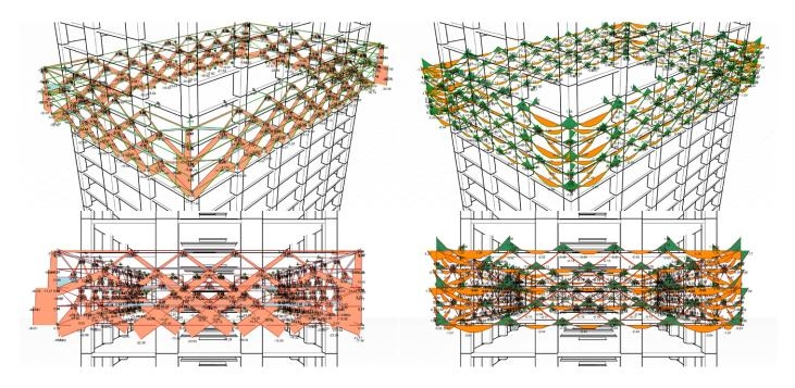
Figure. 87: Axial forces and bending moments calculations with Karamba 3D
