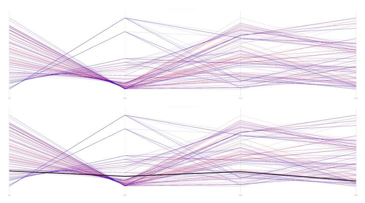
Figure. 93: top fitness objectives parallel coordinate plot where FO1=O1 is the total mass, FO2=O2 is the maximum displacement, FO3=O3 are the cooling demands, FO4=O4 is the average daylight, bottom the highlight of the average fitness ranked solution (the one that is not perfect nor worse for all objectives at the same time)
