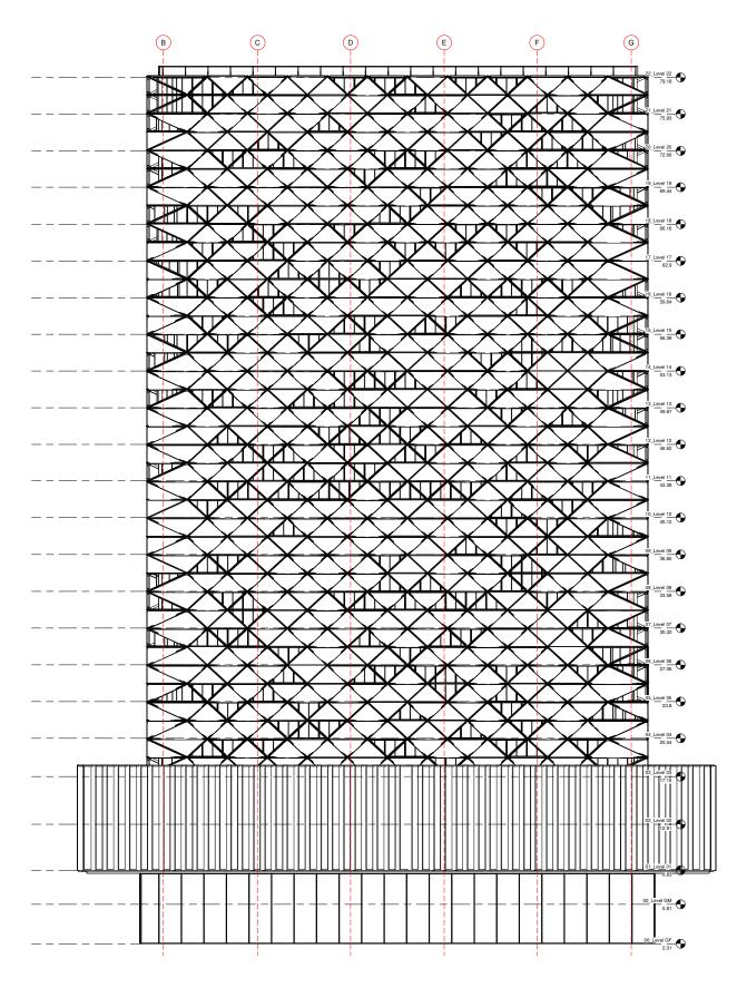
Figure. 115: East facade with proposed shading system
