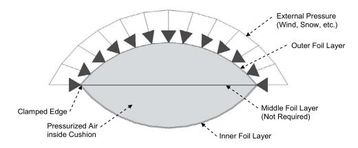
Figure. 13: Schematic ETFE cushion panel (Charbonneau et al., 2014b)
