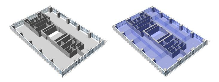
Figure. 56: Main geometry and rooms filtered out from Revit
