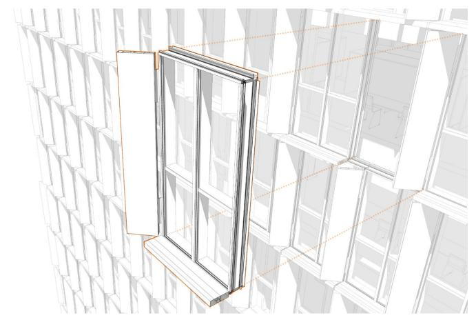
Figure. 45: Typical panel with its horizontal and vertical fins. Drawings by Alkiviadis Oikonomdis based on provided drawings by Eckersley O'Callaghan
