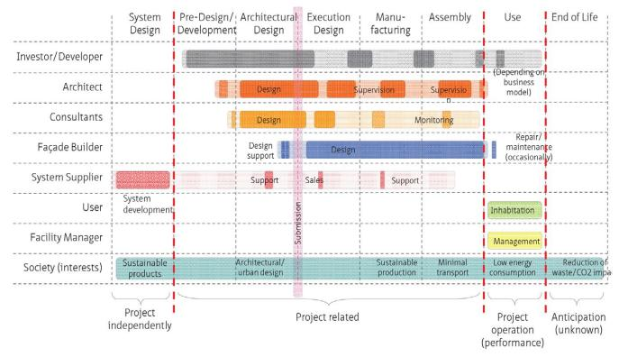
Figure. 6: The different disciplines and roles in façade design (Klein, 2013)
