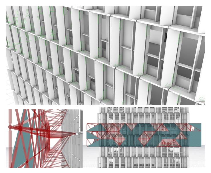
Figure. 75: Brackets connecting the horizontal and vertical fins and first approaches for the shading system.
