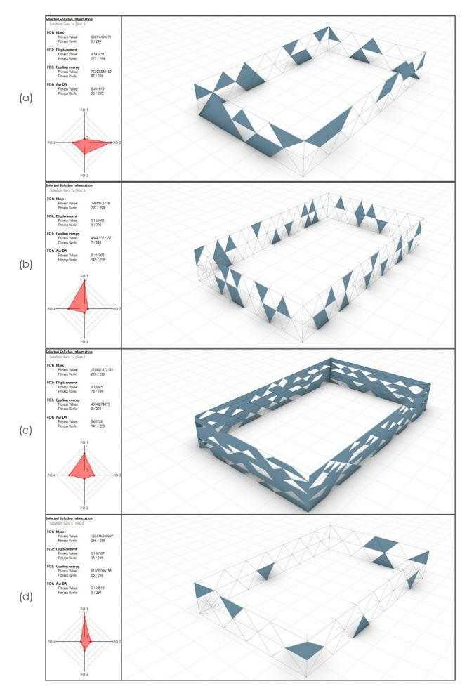
Figure. 97: Extreme solutions: a. best solution for minimal cooling demands, b. best solution for average daylight autonomy of the spaces, c. best solution for minimal mass, d. best solution for minimal displacement
