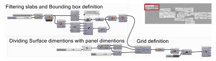
Figure. 77: Isolation of slabs and grid definition
