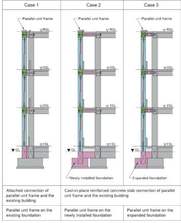
Figure. 109: Different ways of connecting exoskeleton structures on reinforced concrete (Takeda et al,2013)
