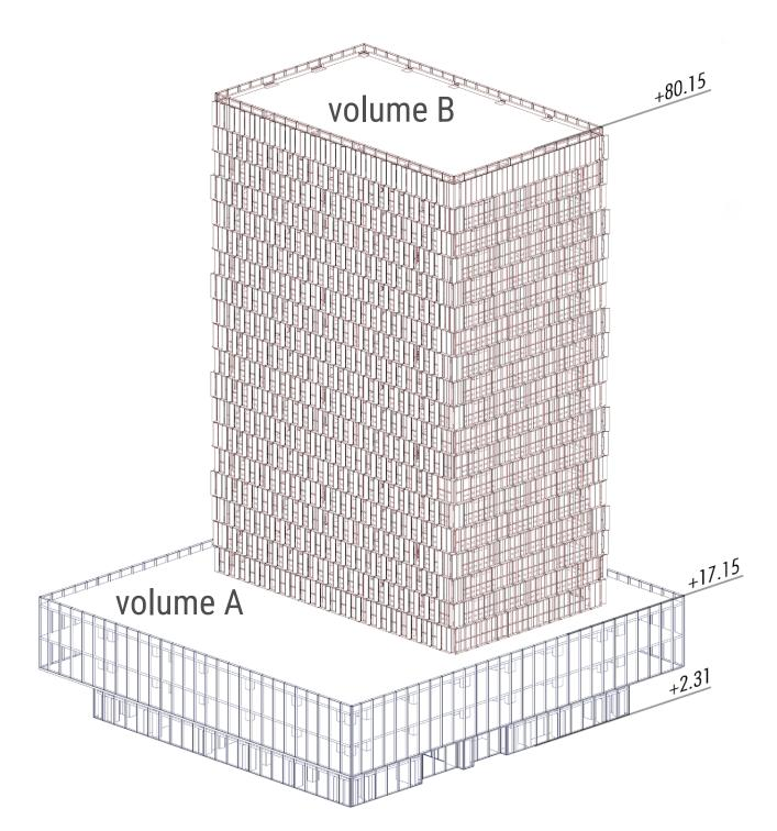
Figure. 35: Piraeus Tower and its main volumes. Design by Alkiviadis Oikonomidis based on the protoype drawings provided by Eckersley O'Callaghan
