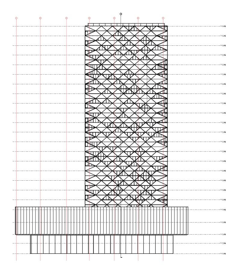
Figure. 118: South facade with proposed shading system
