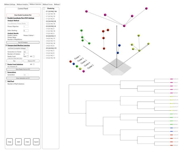
Figure. 94: left Wallacei analysis tab, right Hierarchical solution grouping (complete linkage) with visualiziation in solution space (top) and with a dendrogram (bottom)
