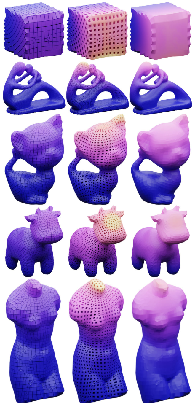
Figure 10: Objects listed in Table 1 as a (solid) hexahedral mesh on the left, corresponding beam and wall micro-structure designs with \alpha = \frac{1}{2} in the centre and on the right, respectively. Colour encodes deformation under load, normalized for visualization.
