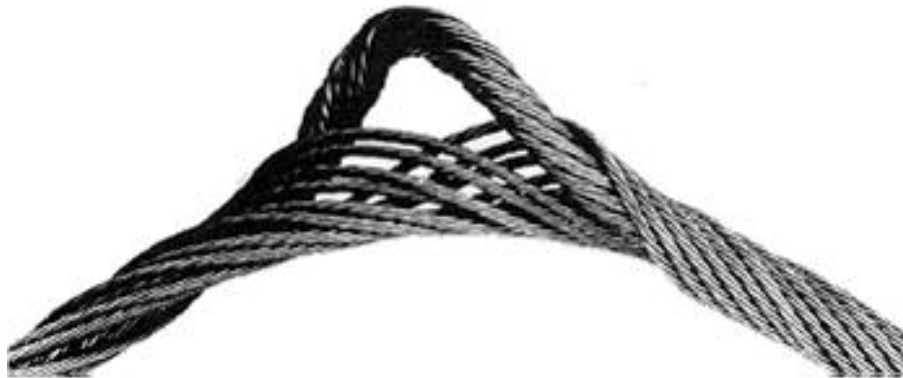
Figure 12: Example of birdcaging a.k.a core protrusion.
