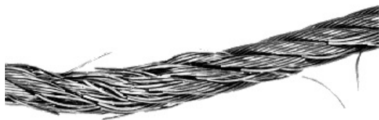
(a) Fatigue failure initiated because the wire rope that ran over an undersized sheave.
