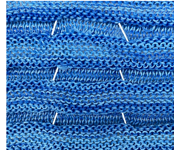
Figure 5.7 Elastic inlay in zig-zag pattern inside ALT design
