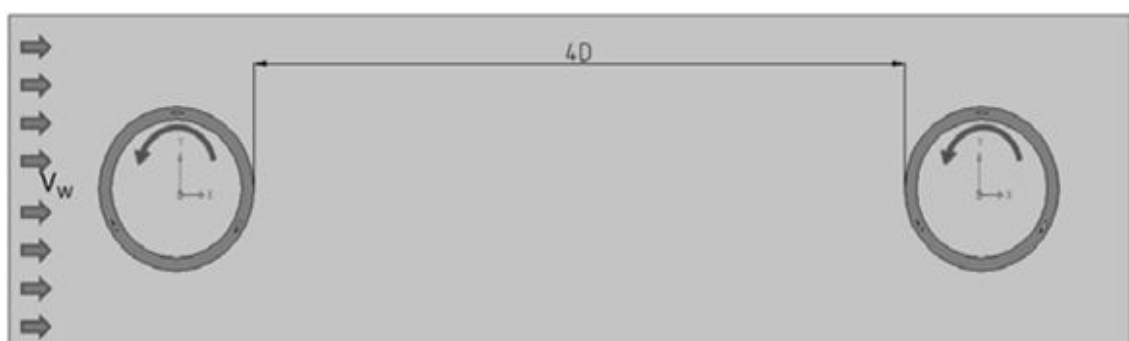
Figure 2.8: Two VAWTs placed in line with a horizontal distance of 4 times the diameter (I-type)
