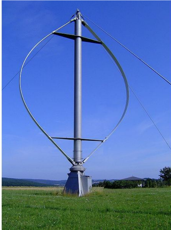
Figure 1.7: A Darrieus wind turbine (Makcan Resources Corporation, 2015)
