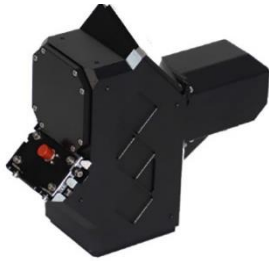
Figure 3.5: An example of a portable IRIS echelle Raman spectrometer (Source: Spectral industries, 2020).
