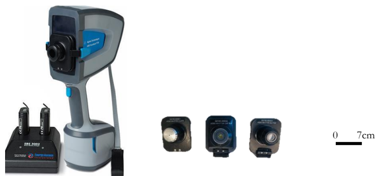
Figure 8.2: Handheld FTIR 4300 spectrometer and the three sampling interfaces.
