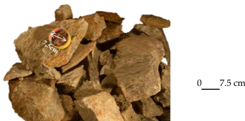
Figure 6.5: An example of an RGB image of a muck pile with known scale reference. This image shows the size of rock fragments at one of the muck pile site.
