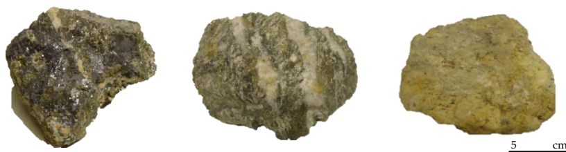
Figure 10.1: Some of the analysed rock chip samples, (a) ore that consists of the sulphide minerals (e.g., galena, pyrite and sphalerite); (b) host rock—banded gneiss; and (c) the weathered material (e.g., clay minerals).
