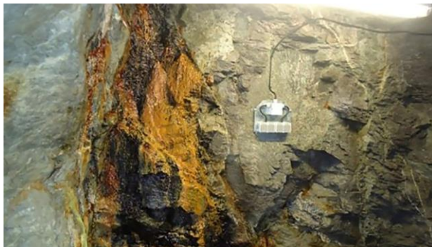
Figure 13.10: A picture that shows surface oxidation at the mine face in an underground mine.
