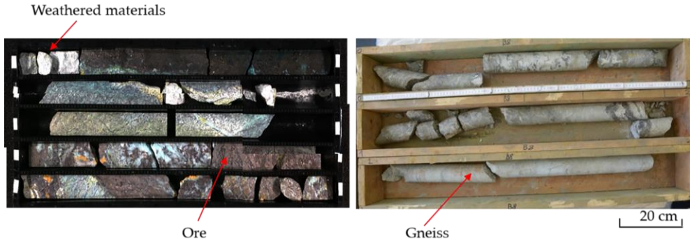
Figure 5.11: Images of drill core samples showing the different lithotypes at the drilled sites. The major lithotypes include the weathered materials (e.g., clay minerals), the ore that consists of the sulphide minerals and host rock (gneiss).
