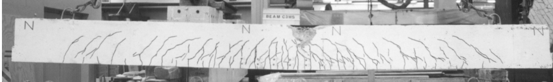
Figure 7.15 ULS crack pattern beam C3 north face
