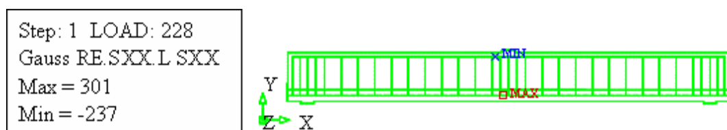
Figure 9.26 Maximum and minimum stresses in reinforcement components at SLS load level on beam B2
