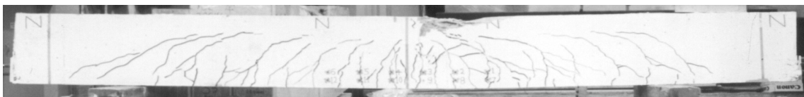
Figure 8.24 Crack pattern at failure load in experiment B2
