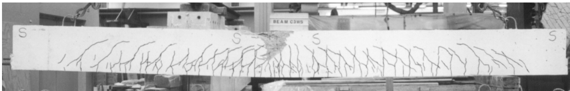
Figure 7.15 ULS crack pattern beam C3 north face
