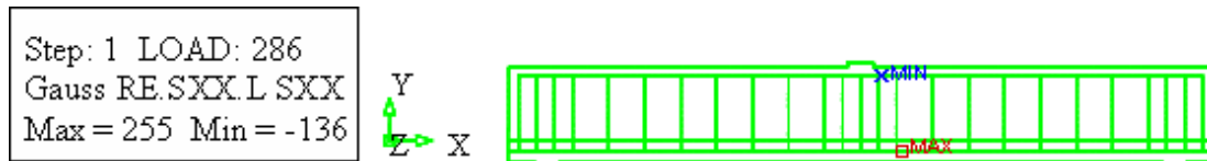
Figure 9.14 Stress reinforcement at SLS load level.
